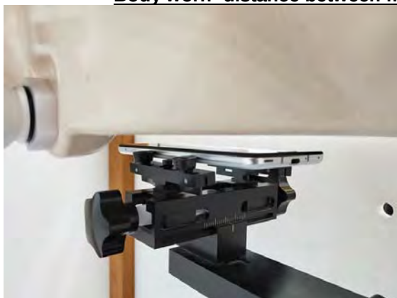
Fig.7 EUT Front side to flat phantom
