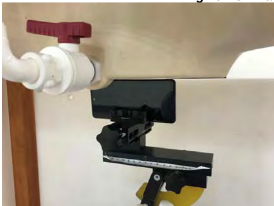
Fig.17 EUT Right side to flat phantom
