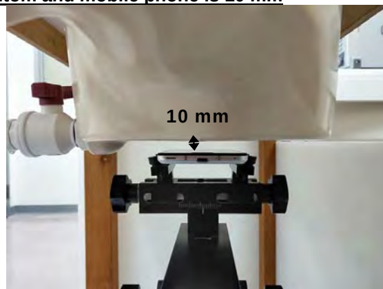
Fig.7 EUT Front side to flat phantom
