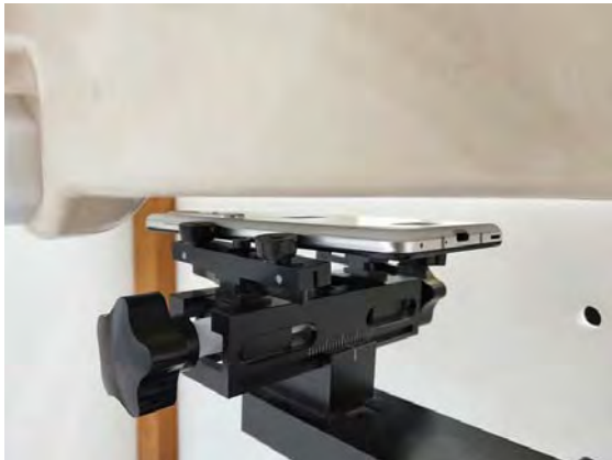
Fig.10 EUT Back side to flat phantom
