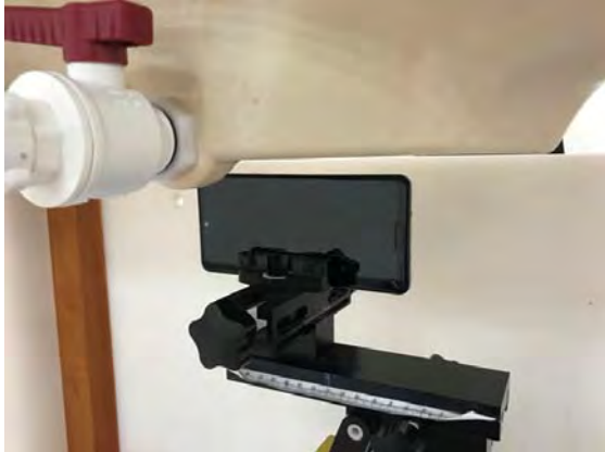
Fig.12 EUT Right side to flat phantom
