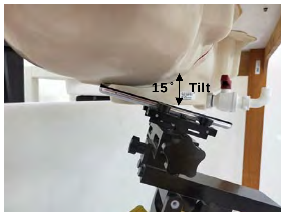
Fig.4 Right Head Section / Ear-Tilt Position(15°)
