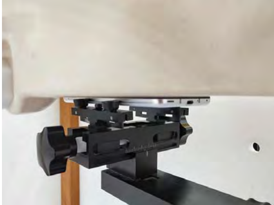
Fig.15 EUT Front side to flat phantom
