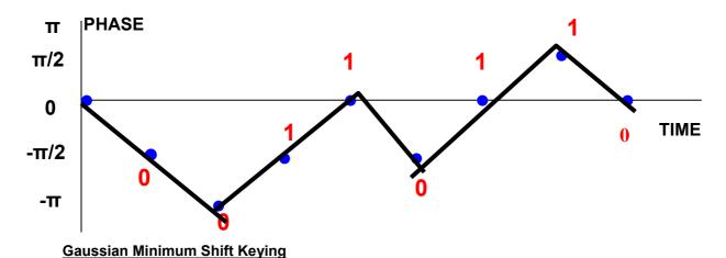
MSK has high sidebands relative to the main lobes in the frequency domain - this can lead to interference with adjacent signals.
