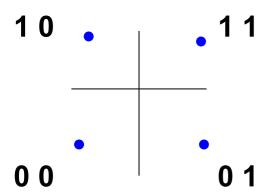
Therefore for the BIT sequence 0 0 1 1 1 0 0 1 The corresponding phase shift will be used
