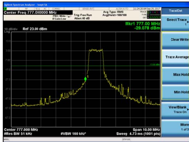
LTE Band 13 16QAM 10MHz CH-Low, 1 RB
