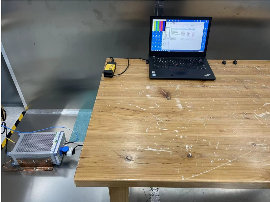
Photograph 3: Set-up for Conducted Emission on AC Mains
