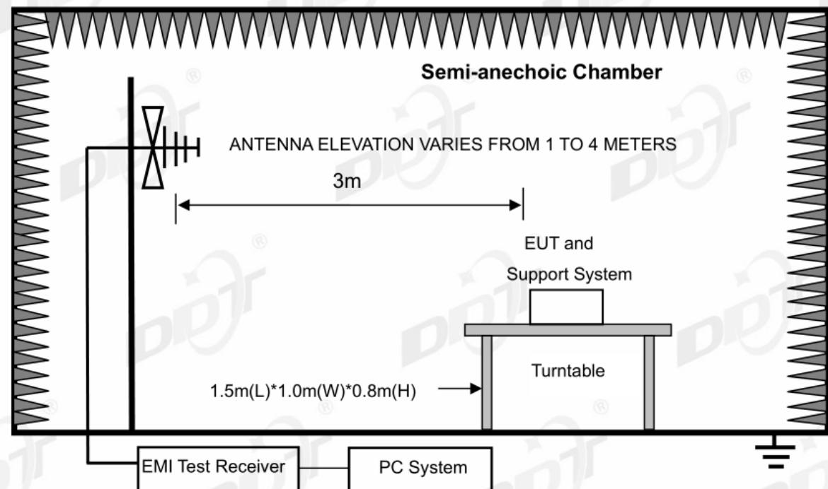
In 3 m Anechoic Chamber, test setup diagram for frequency above 1 GHz:
