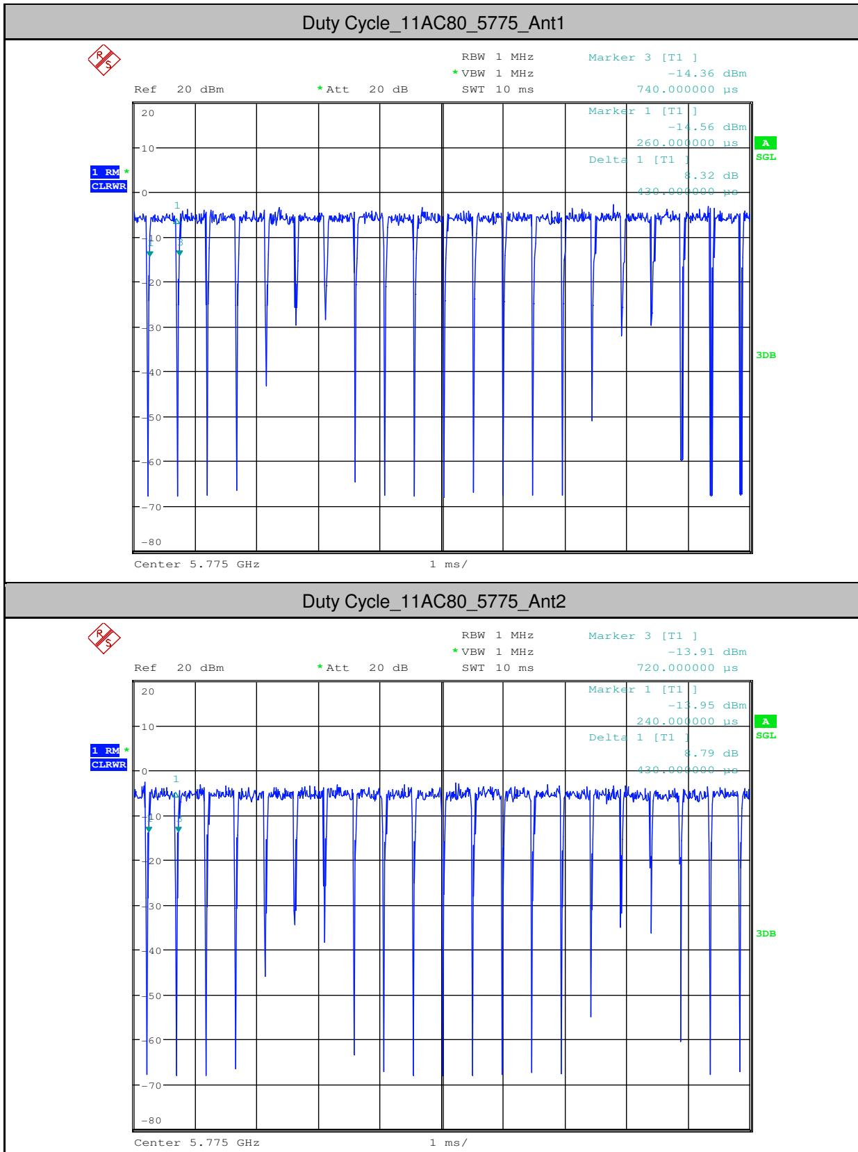
**6. (DFS: Channel Move Time; DFS: Channel Closing Transmission Time)**
