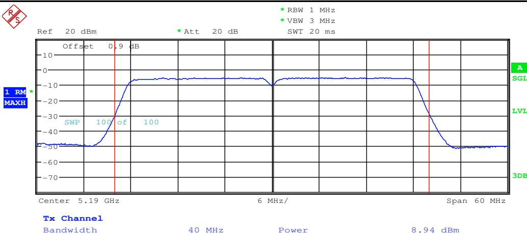
Maximum Conduct Output Power\_11N40\_5230\_Ant1
