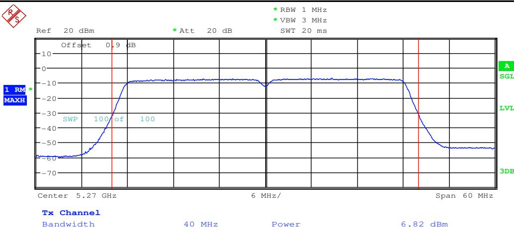
Maximum Conduct Output Power\_11N40\_5310\_Ant1
