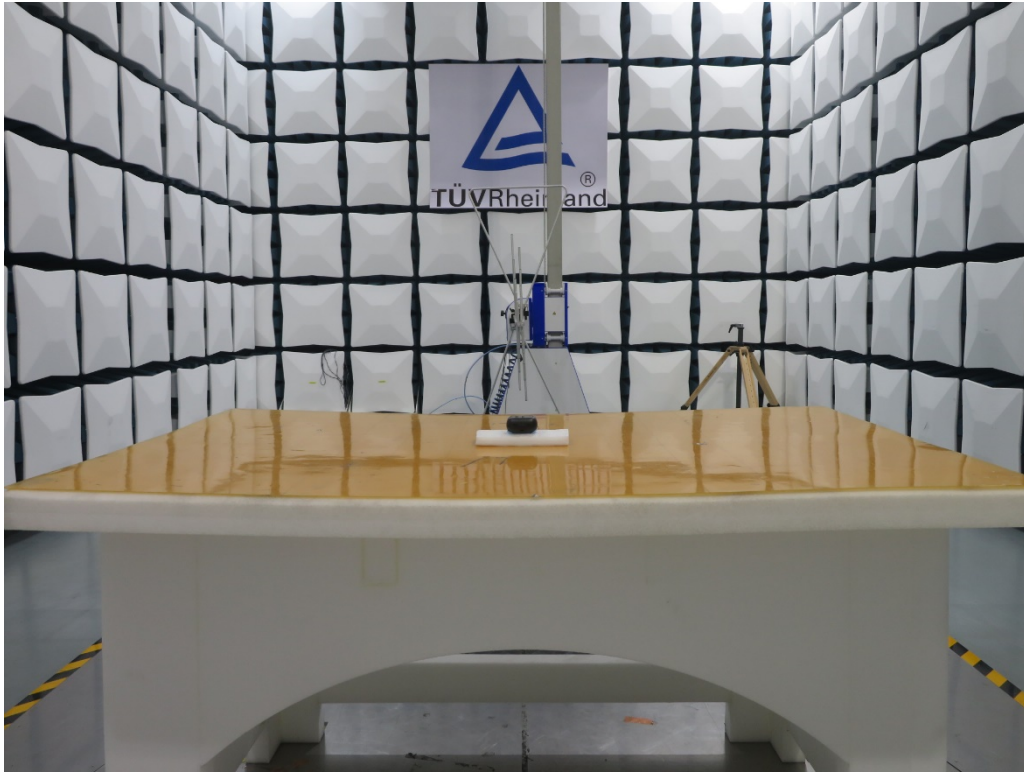
Photograph 1: Set-up for Radiated Spurious Emission, Below 1GHz
