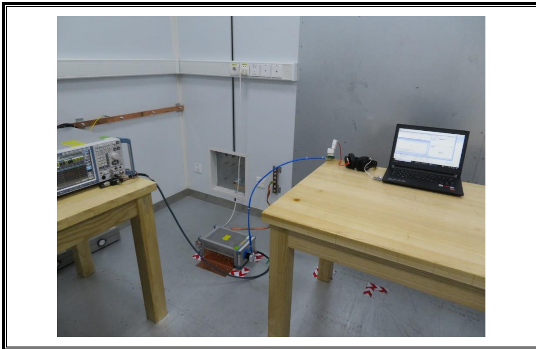
POWERLINE CONDUCTED EMISSIONS MEASUREMENT SETUP
