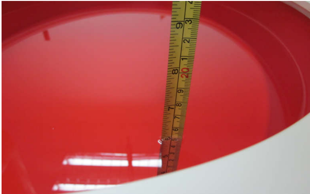
Figure 4.4: Liquid depth in the Flat Phantom
