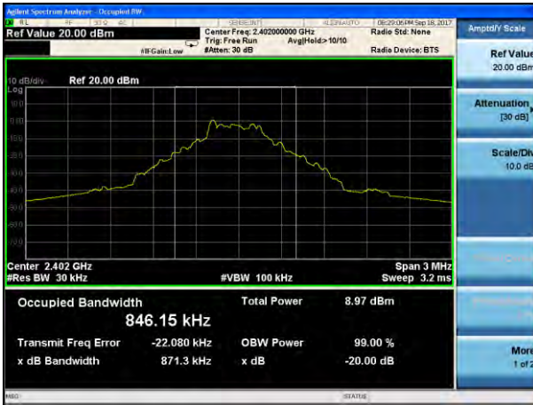
20dB Bandwidth plot on channel 39 (1Mbps)
