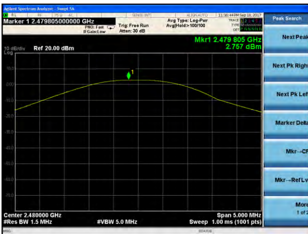
Peak output Power plot on channel 78 (1Mbps)
