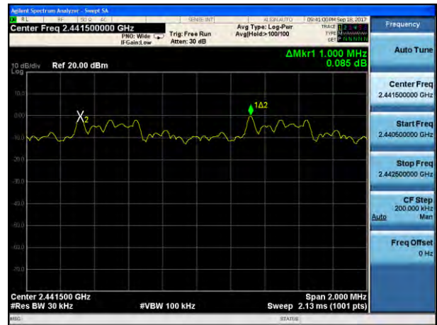
(2Mbps) Channel Separation plot on channel 77-78
