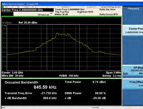
20dB Bandwidth plot on channel 78 (1Mbps)
