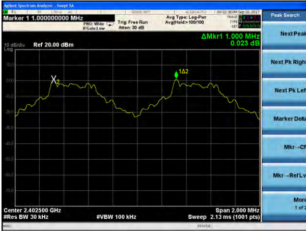
(1Mbps) Channel Separation plot on channel 39-40
