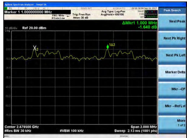
(2Mbps) Channel Separation plot on channel 77-78
