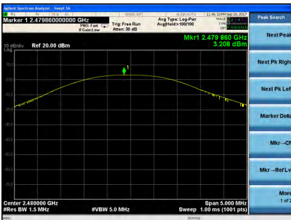
Peak output Power plot on channel 78 (3Mbps)
