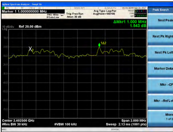
(3Mbps) Channel Separation plot on channel 39-40
