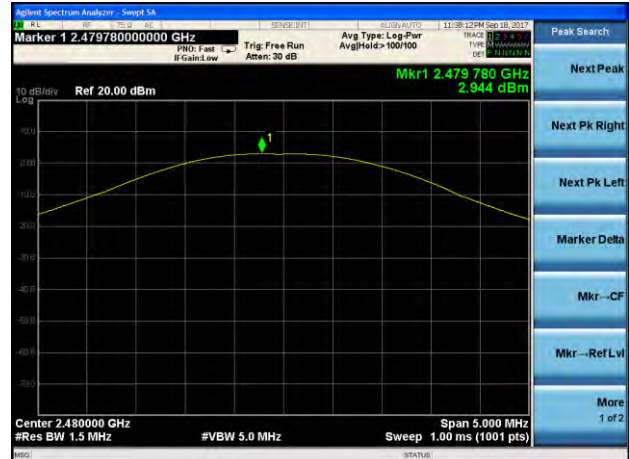
Peak output Power plot on channel 78 (2Mbps)
