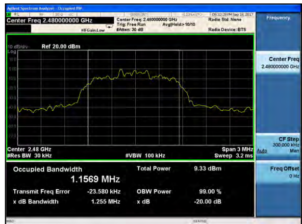
20dB Bandwidth plot on channel 78 (2Mbps)
