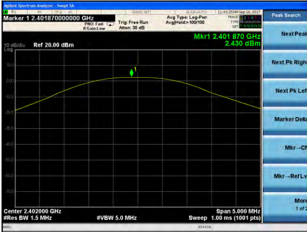
Peak output Power plot on channel 39 (3Mbps)
