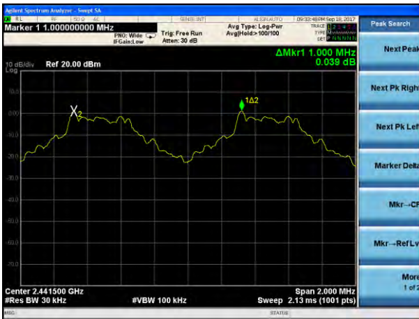
(1Mbps) Channel Separation plot on channel 77-78
