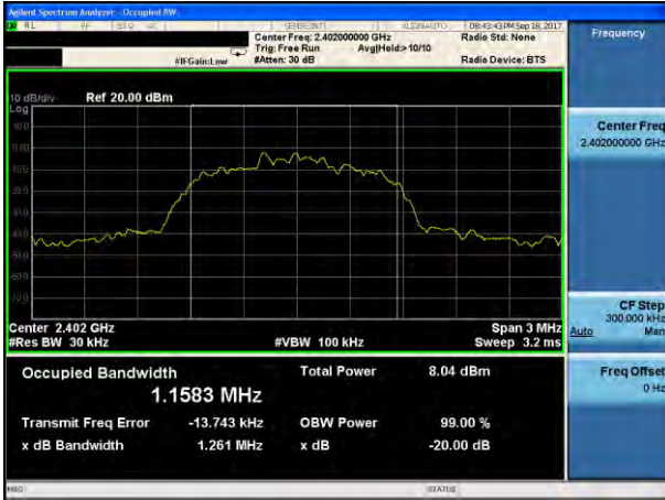
20dB Bandwidth plot on channel 39 (3Mbps)
