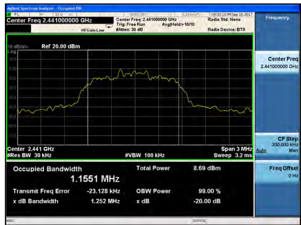
20dB Bandwidth plot on channel 39 (2Mbps)
