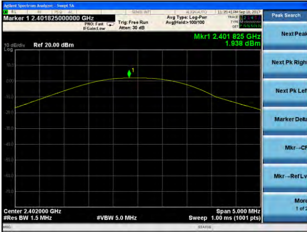
Peak output Power plot on channel 39 (1Mbps)
