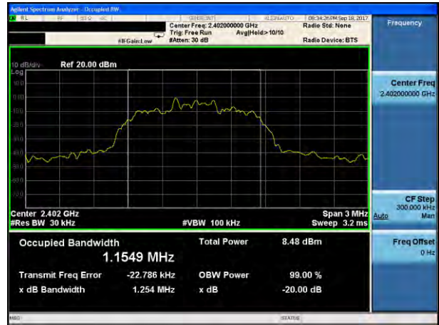
20dB Bandwidth plot on channel 39 (2Mbps)
