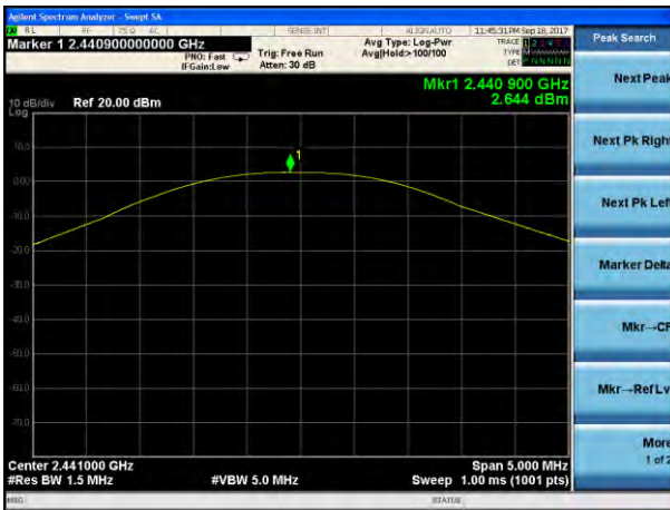
Peak output Power plot on channel 39 (3Mbps)
