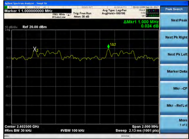
(2Mbps) Channel Separation plot on channel 39-40
