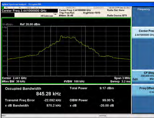
20dB Bandwidth plot on channel 39 (1Mbps)
