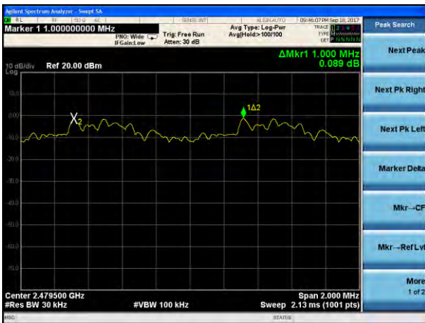
(3Mbps) Channel Separation plot on channel 77-78
