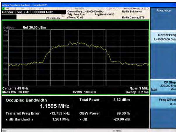
20dB Bandwidth plot on channel 78 (3Mbps)
