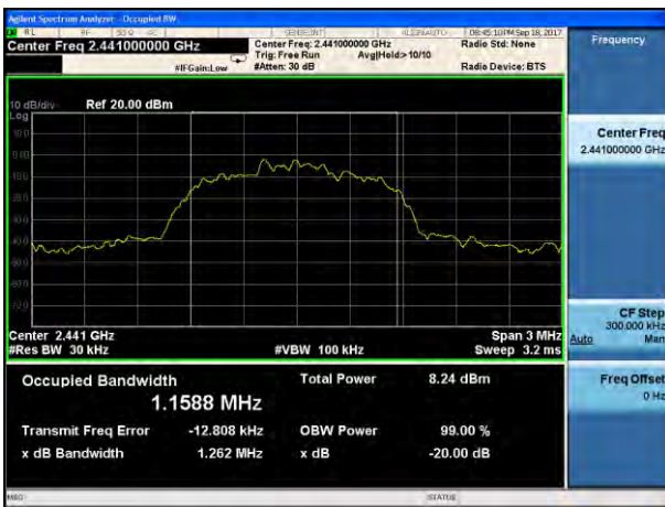
20dB Bandwidth plot on channel 39 (3Mbps)
