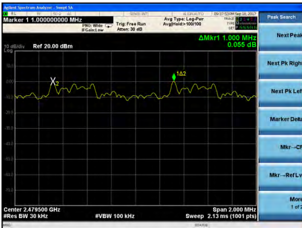
(1Mbps) Channel Separation plot on channel 77-78
