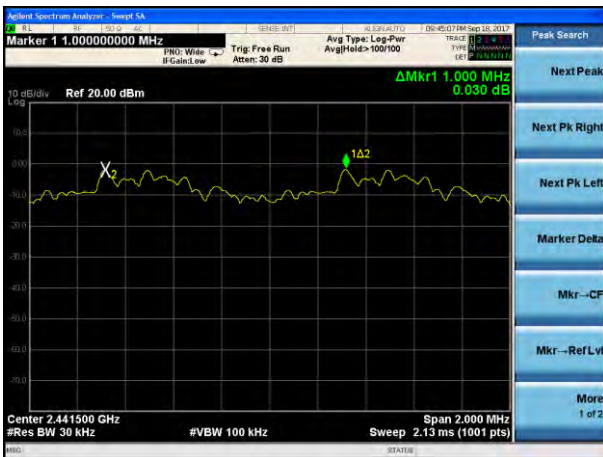
(3Mbps) Channel Separation plot on channel 77-78
