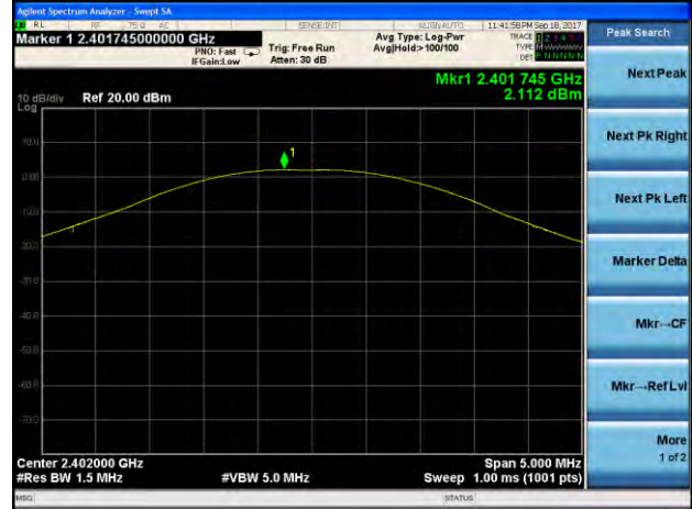
Peak output Power plot on channel 39 (2Mbps)
