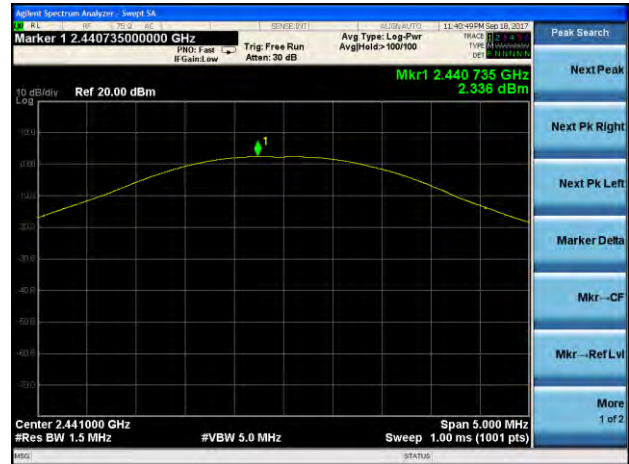
Peak output Power plot on channel 78 (2Mbps)
