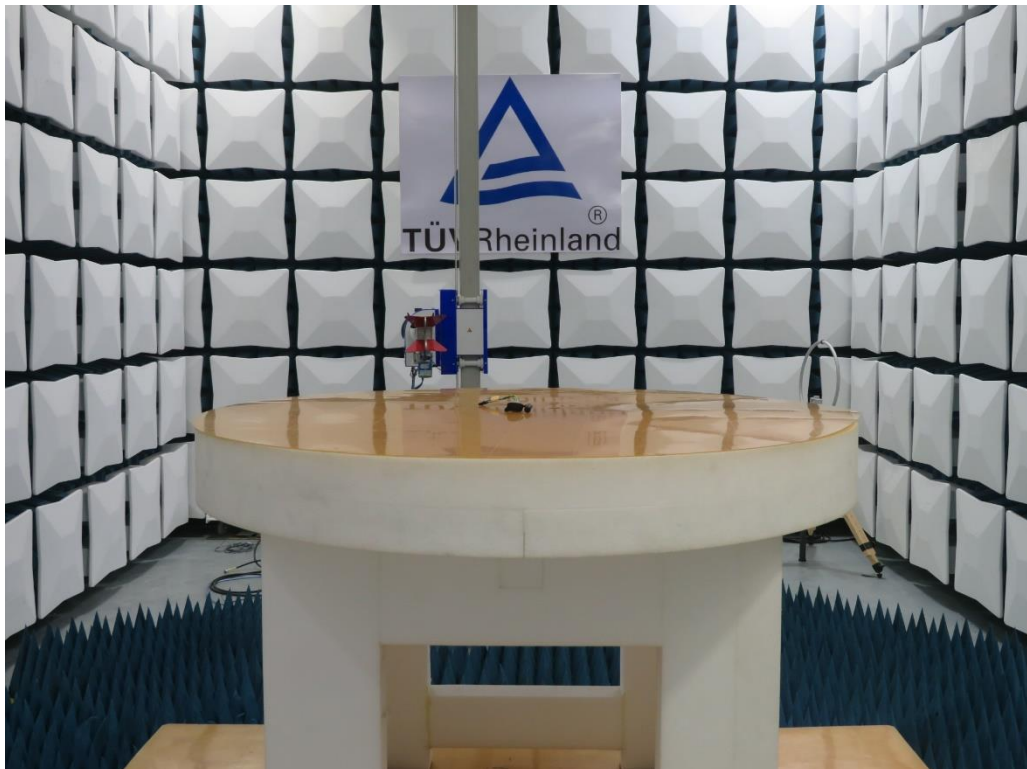
Photograph 2: Set-up for Radiated Spurious Emission, Above 1GHz
