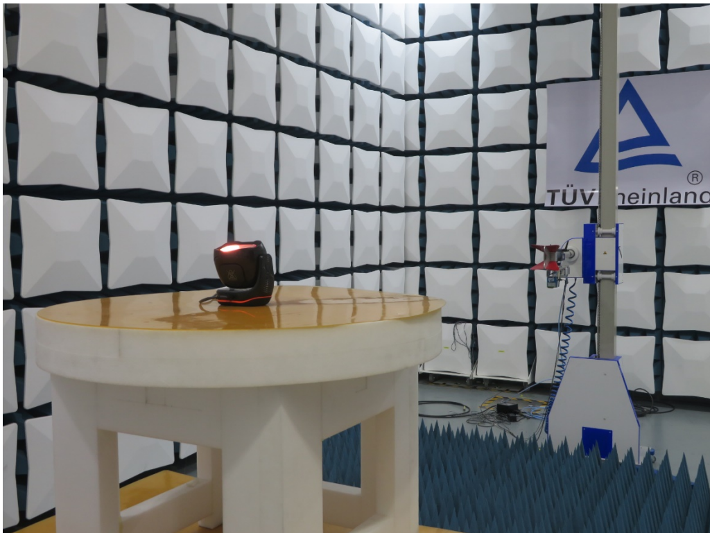
Photograph 2: Set-up for Radiated Spurious Emission, Above 1GHz
