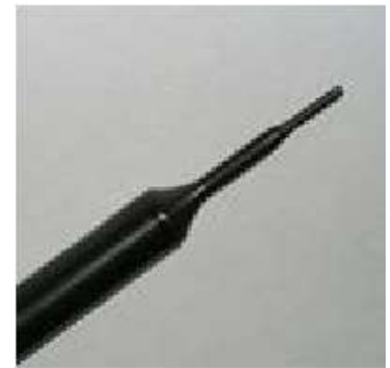
Figure 4.4 EX3DV4 E-field Probe
