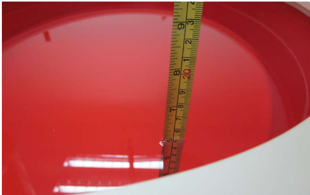
Figure 4.4: Liquid depth in the Flat Phantom
