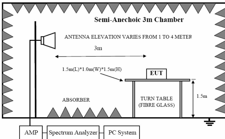
Note: For harmonic emissions test a appropriate high pass filter was inserted in the input port of AMP.
