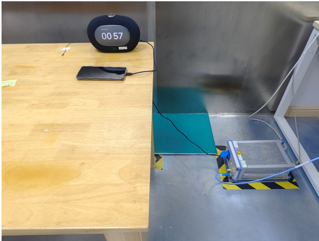
Photograph 3: Set-up for Conducted Emission on AC Mains
