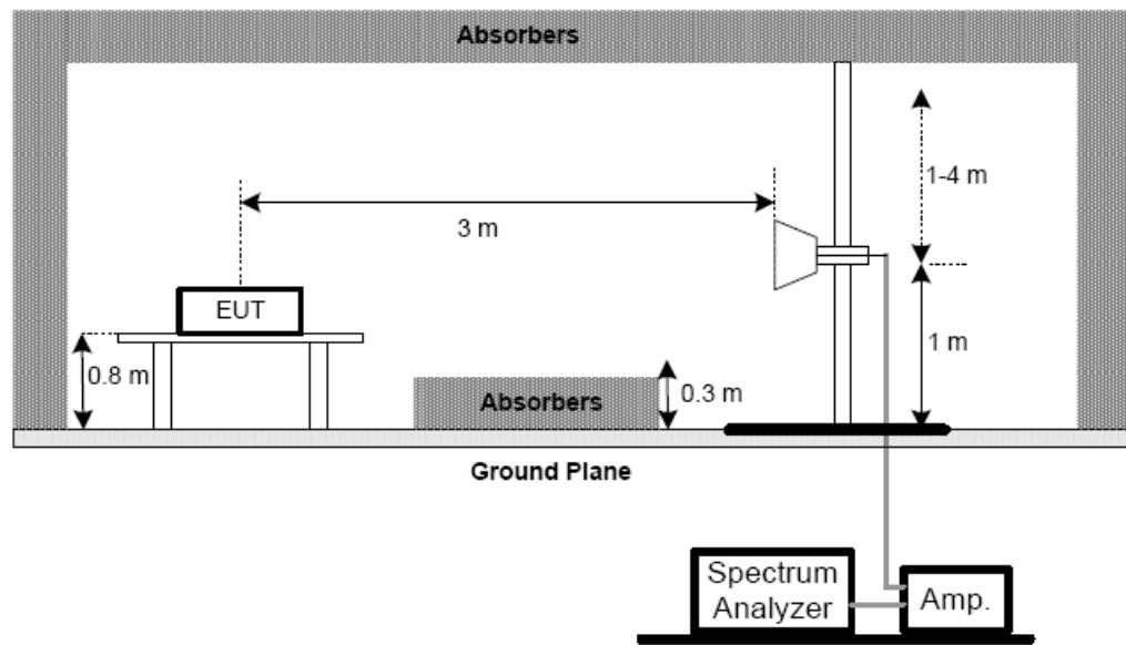
(C) For radiated emissions below 30MHz
