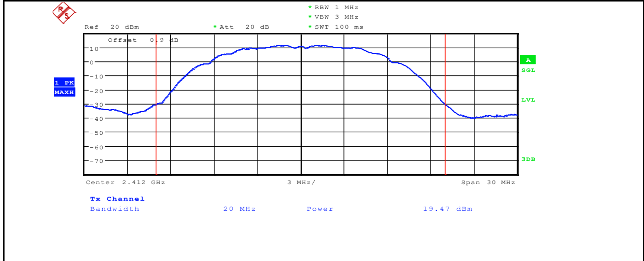
Maximum peak conducted output power_11B_2437
