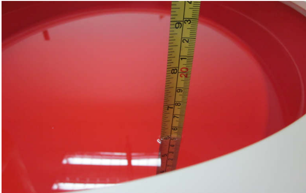
Figure 4.4: Liquid depth in the Flat Phantom
