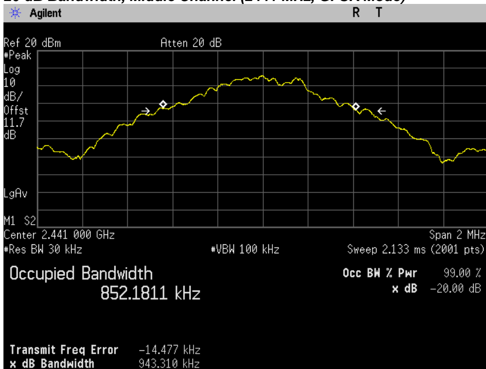
20 dB Bandwidth, Middle Channel (2441 MHz, GFSK Mode)
