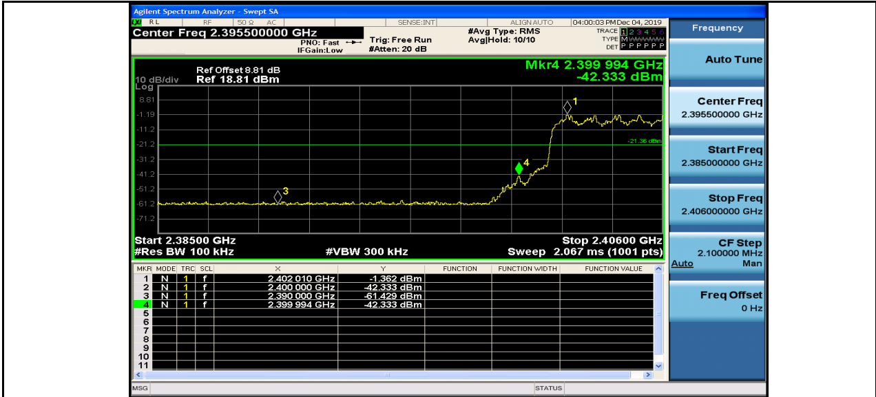
Band-edge for RF Conducted Emissions_3DH5_2402_Hopping Off
