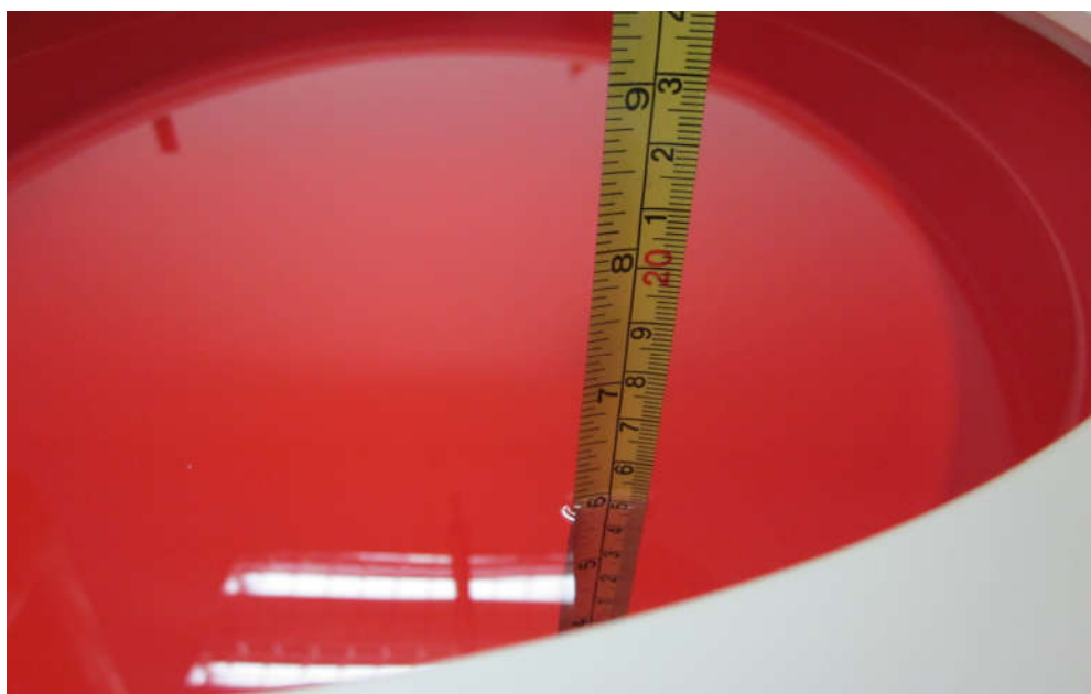
Figure 4.4: Liquid depth in the Flat Phantom
