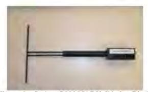
Figure 1 - Satimo COMOSAR Validation Dipole
