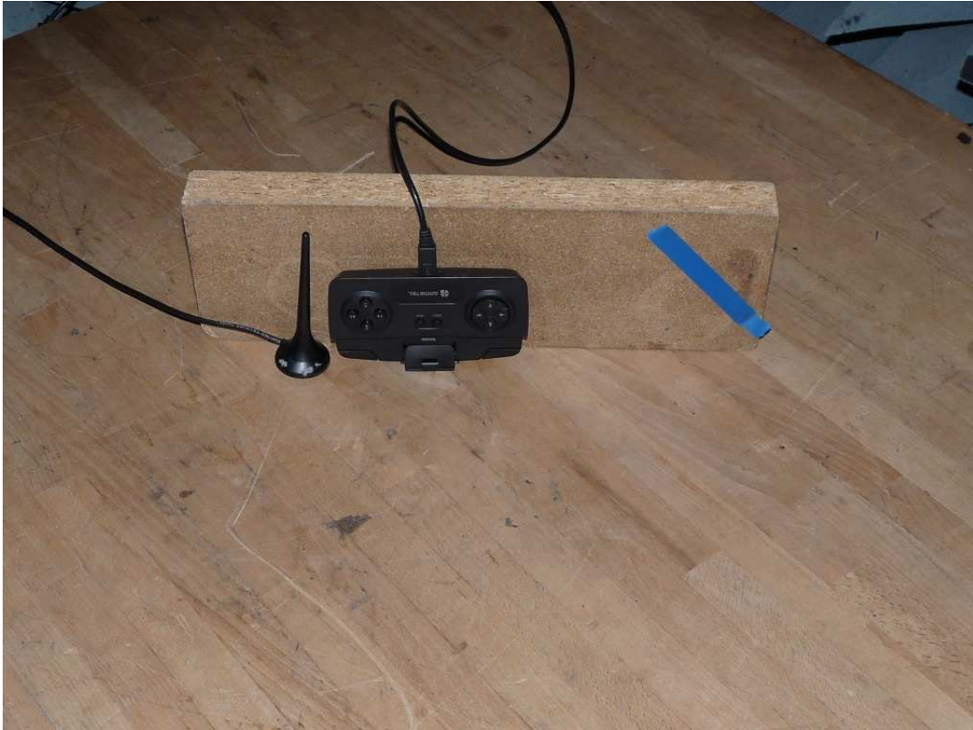
Photo 1: Test setup for radiated measurements (below 30 MHz)
