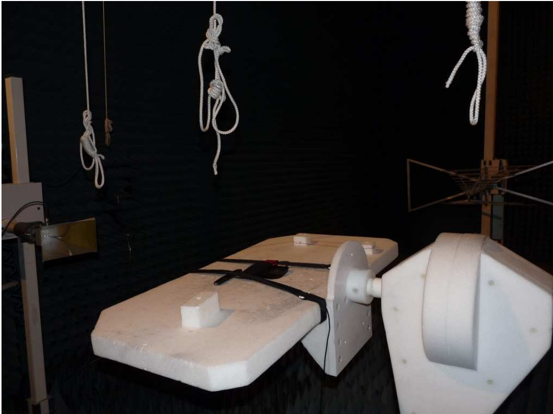
Photo 5: Test setup for radiated measurements (above 18 -25 GHz)
