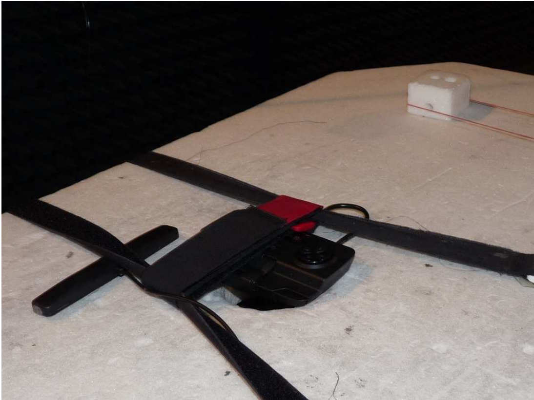
Photo 4: Test setup for radiated measurements (above 1 -18 GHz)
