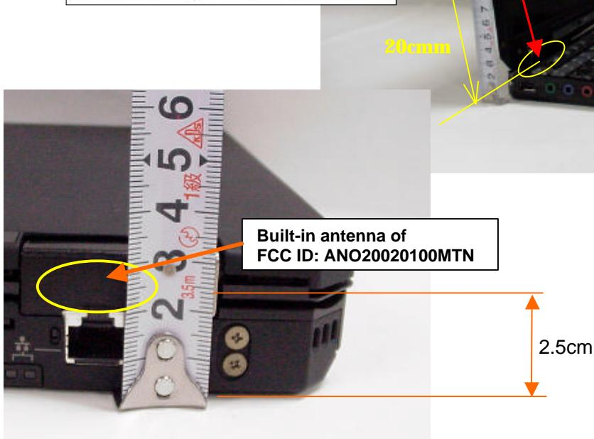
The main and auxiliary antennas placed at LCD section of the each host device (ThinkPad T40 Series, or X30 Series) are assembled apart from each Bluetooth antenna shown in the previous page with 20 cm or more.
