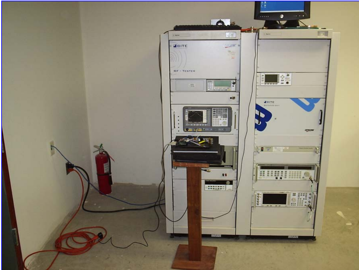
Photograph 2. Output Power; Test Setup
