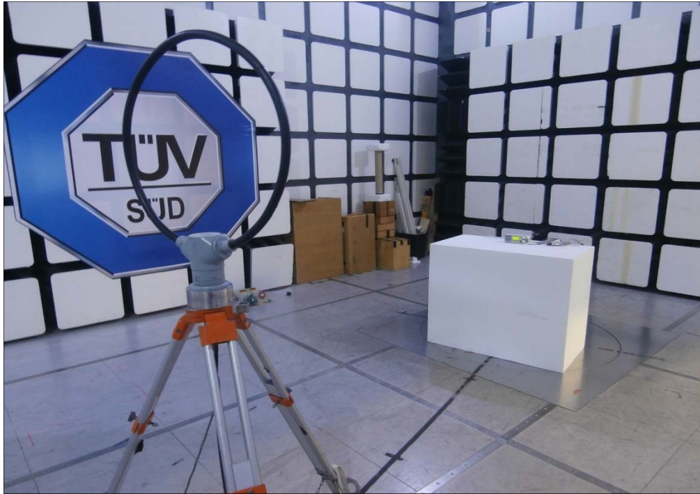
Figure 9 - Test Setup - 9kHz to 30MHz
