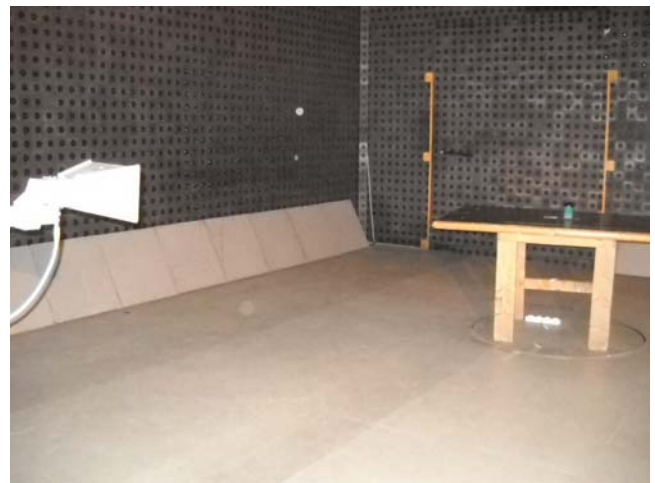
Photograph 8.1.1 Setup for radiated emission measurements
