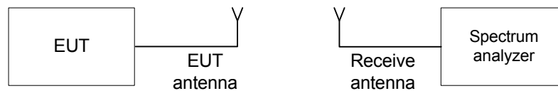
Figure 7.4.1 Occupied bandwidth test setup
