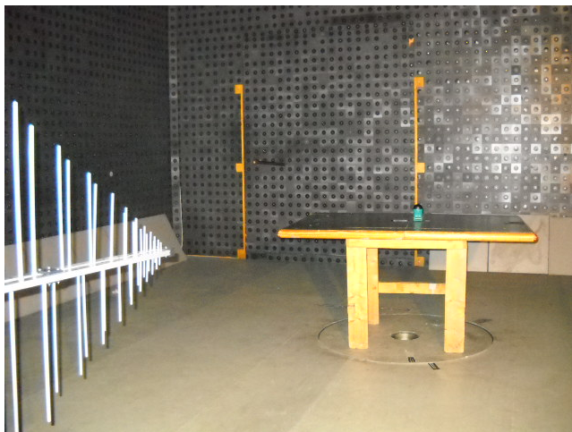
Photograph 8.1.1 Setup for radiated emission measurements
