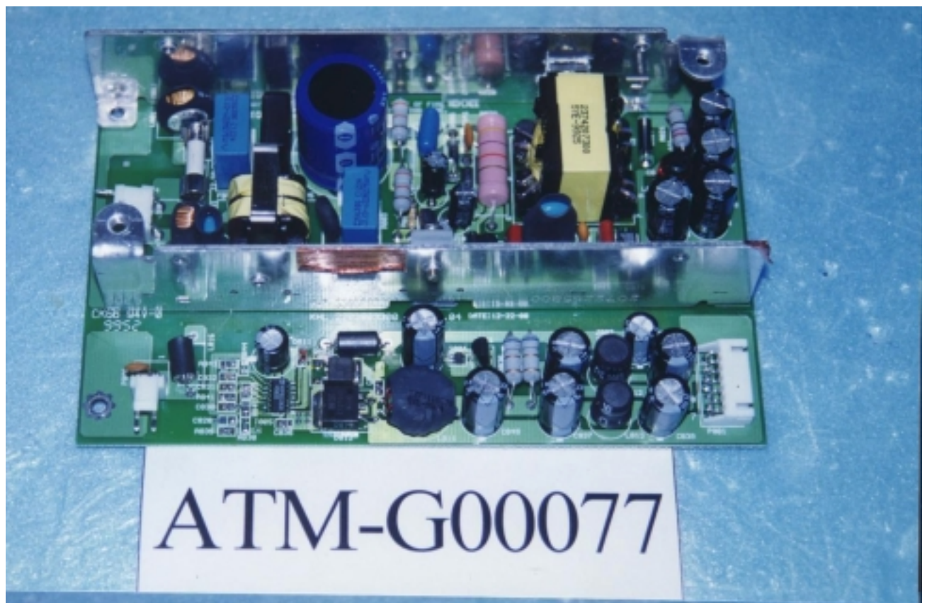
Figure 16 Switching Power Supply
