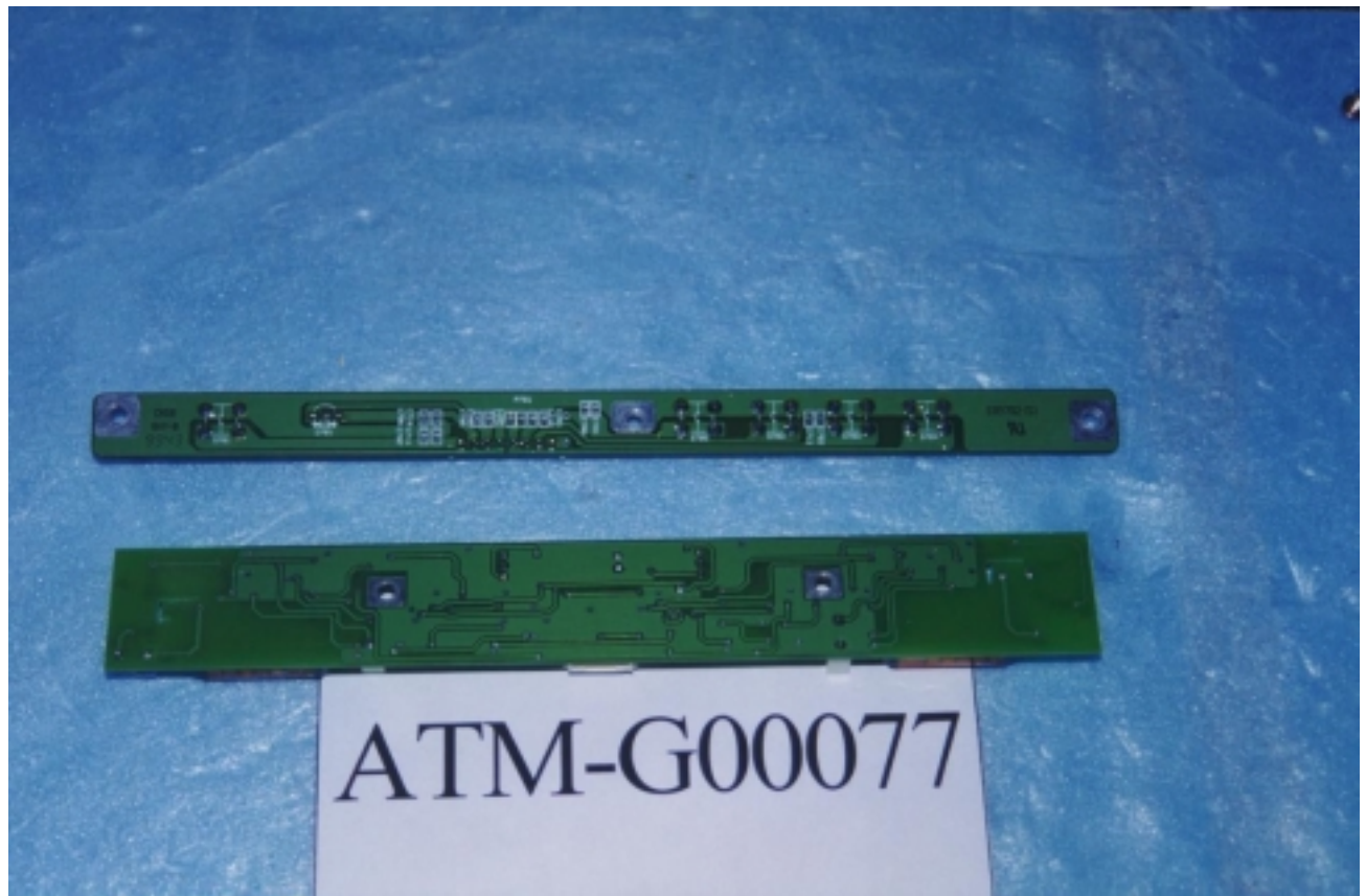
Figure 19 Inverter Board & Button Control Board
