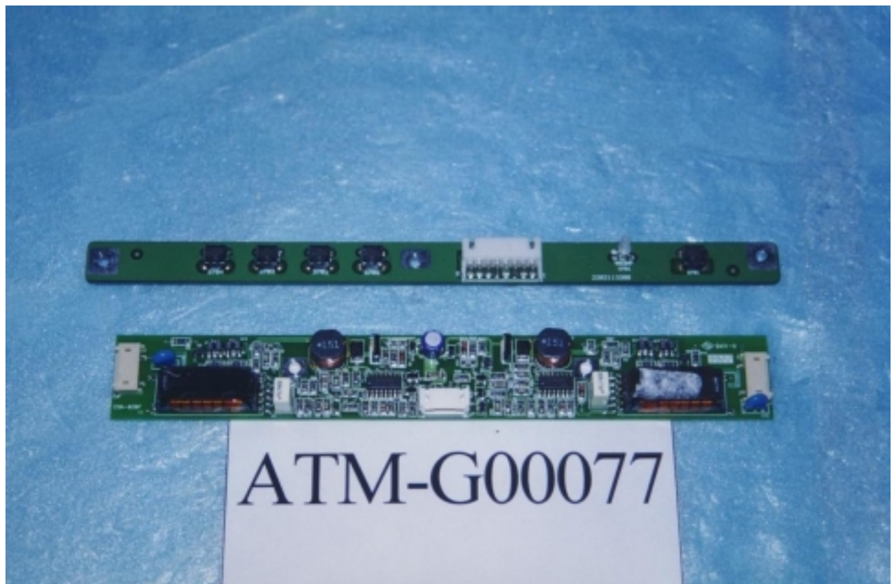
Figure 18 Inverter Board & Button Control Board
