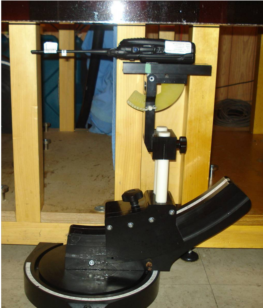
Face-held SAR Configuration Test Setup
