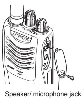
If you are not using a speaker/ microphone, install the cover over the speaker/ microphone jacks using the supplied 3 x 6 mm screw.
