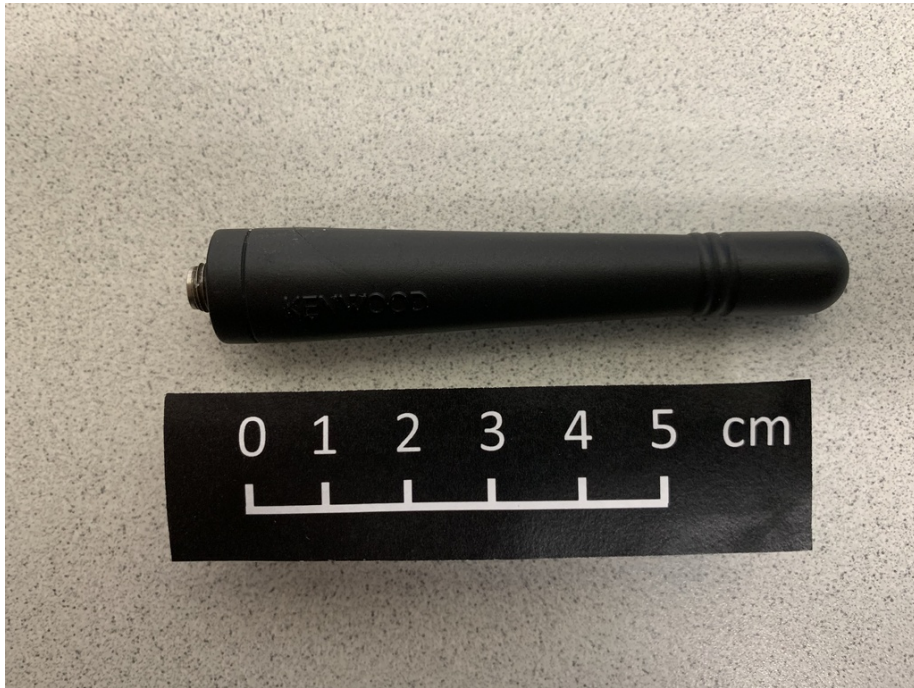
Antenna Model: KRA-23M, Length = 80mm (Antenna P/N T90-0798-x0)
