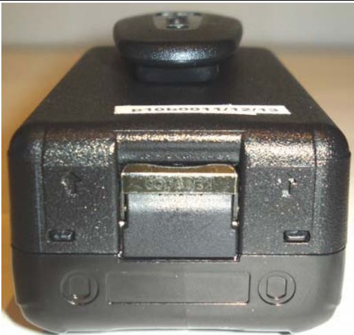
Bottom end of NX-320-K6 w/ KBP-5 Alk Case "Batt d" & Belt-Clip
