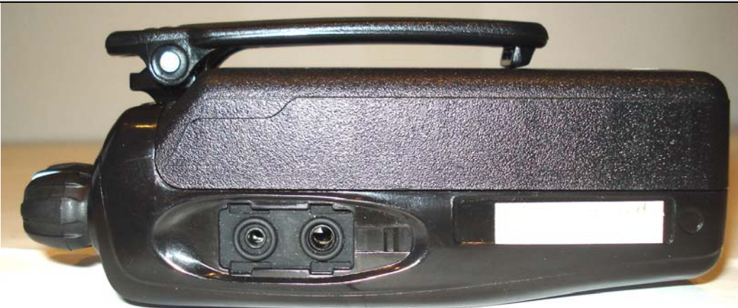
Right Side of NX-320-K6 with KBP-5 Alkaline Case "Battery d" & Belt-Clip accessory
