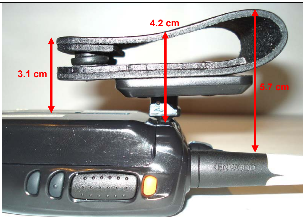
Swivel Belt-Loop measurement distance from Back of DUT & Antenna Base – KNB-57L Li-ion “Battery a”
