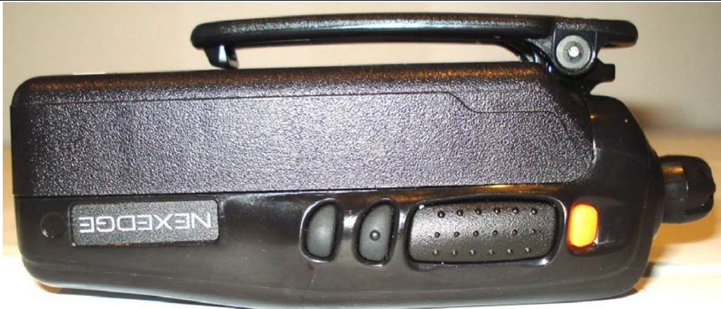
Left Side of NX-320-K6 with KBP-5 Alkaline Case "Battery d" & Belt-Clip accessory
