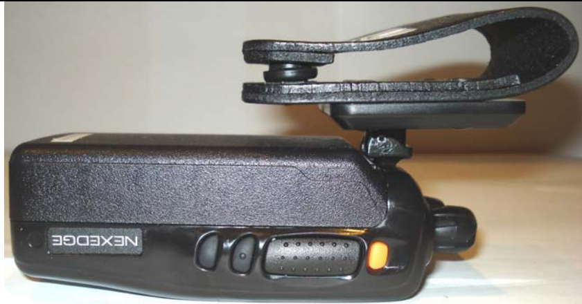
Left Side of NX-320-K6 with KBP-5 Alkaline Case "Battery d" & Swivel Belt-Loop accessory
