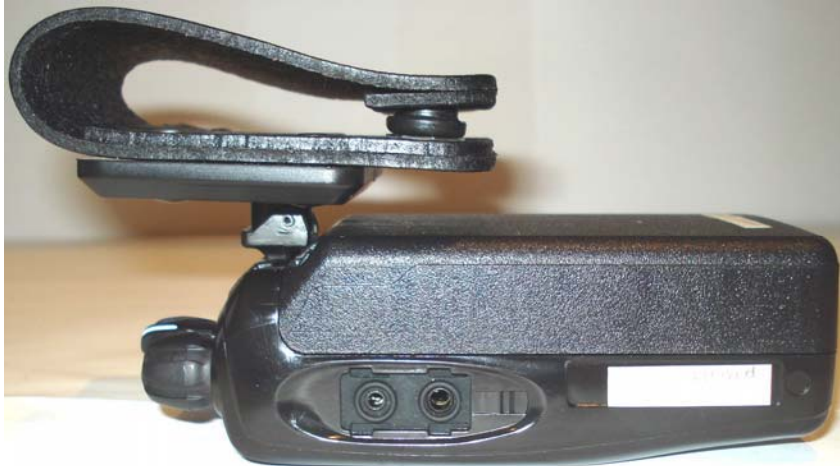
Right Side of NX-320-K6 with KBP-5 Alkaline Case "Battery d" & Swivel Belt-Loop accessory
