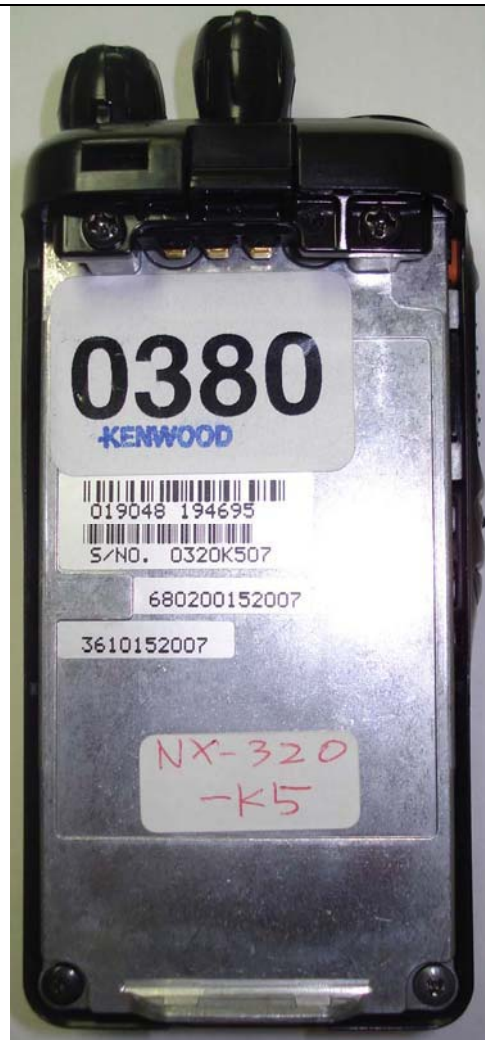
Back of NX-320-K5 with Battery Removed
