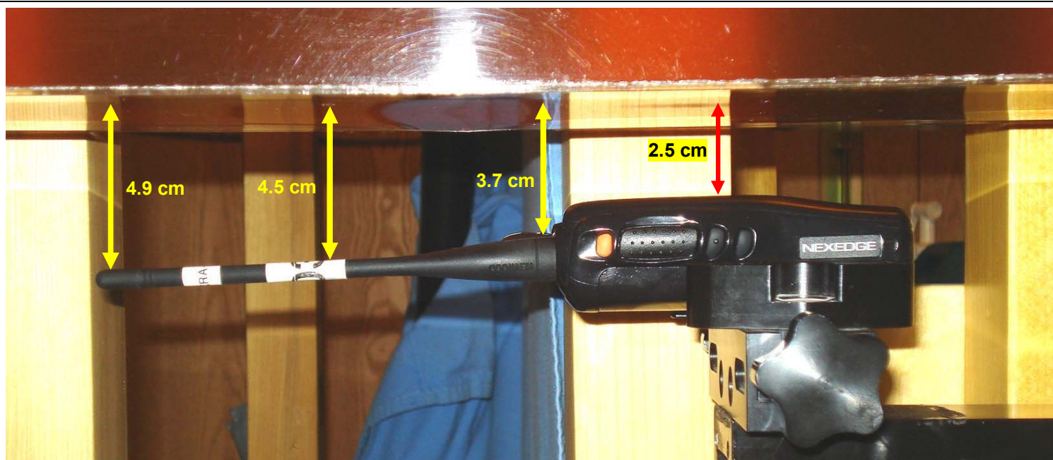
NX-320-K6 with KRA-27M "Antenna C" & KNB-55L Li-ion "Battery (b)"
