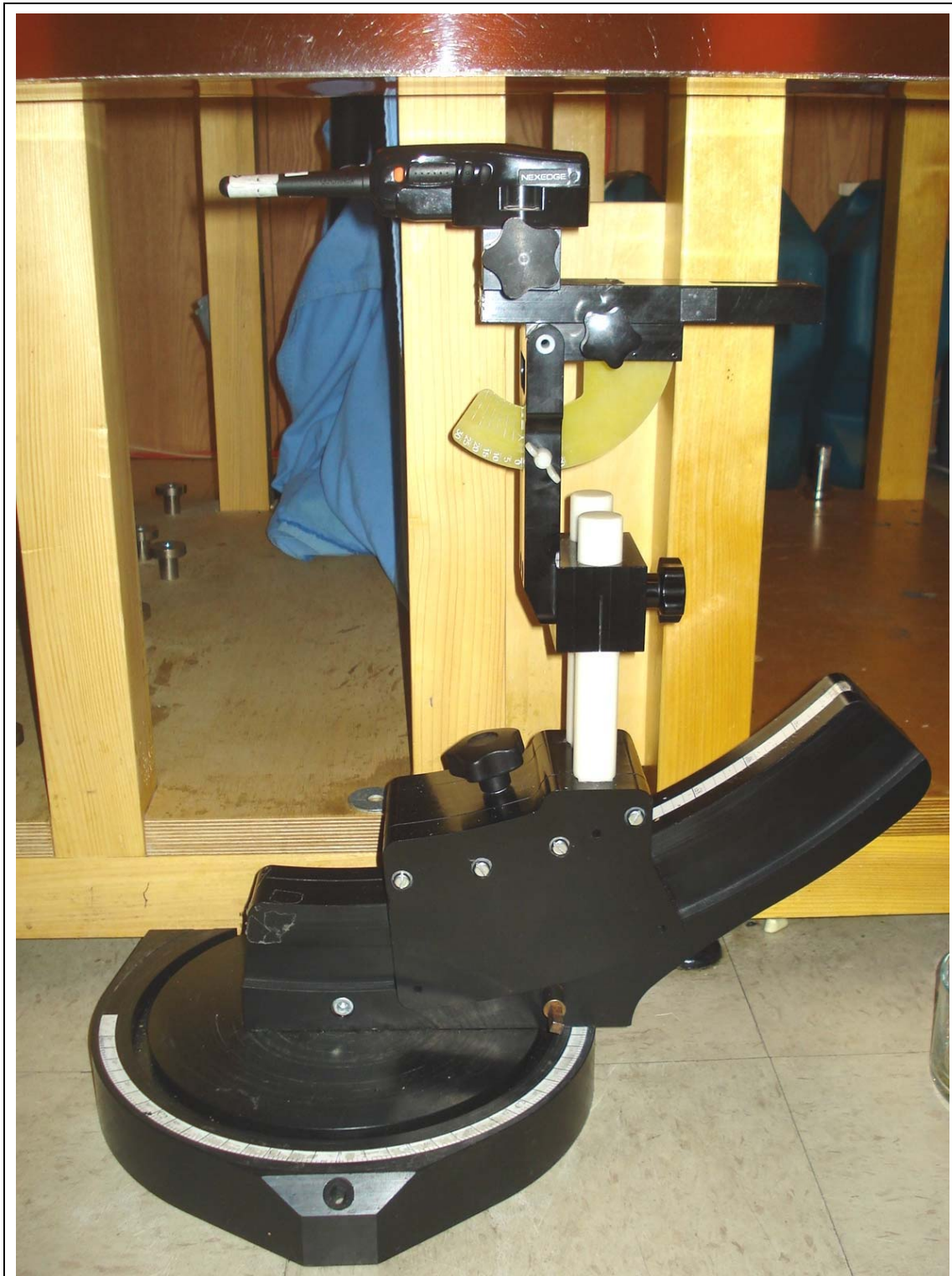
Face-held SAR Configuration Test Setup
