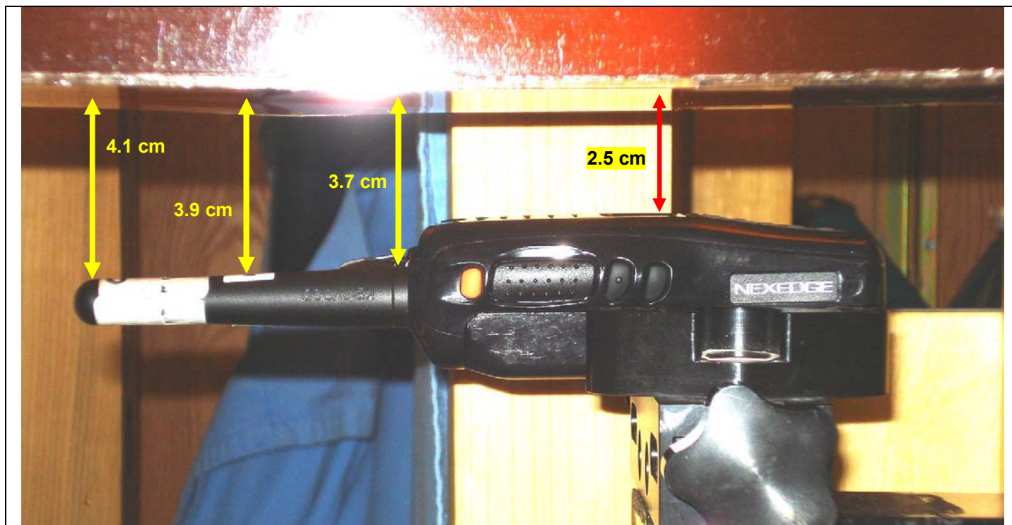
NX-320-K6 with KRA-23M/M3* "Antenna A/B" & KNB-57L Li-ion "Battery (a)"
