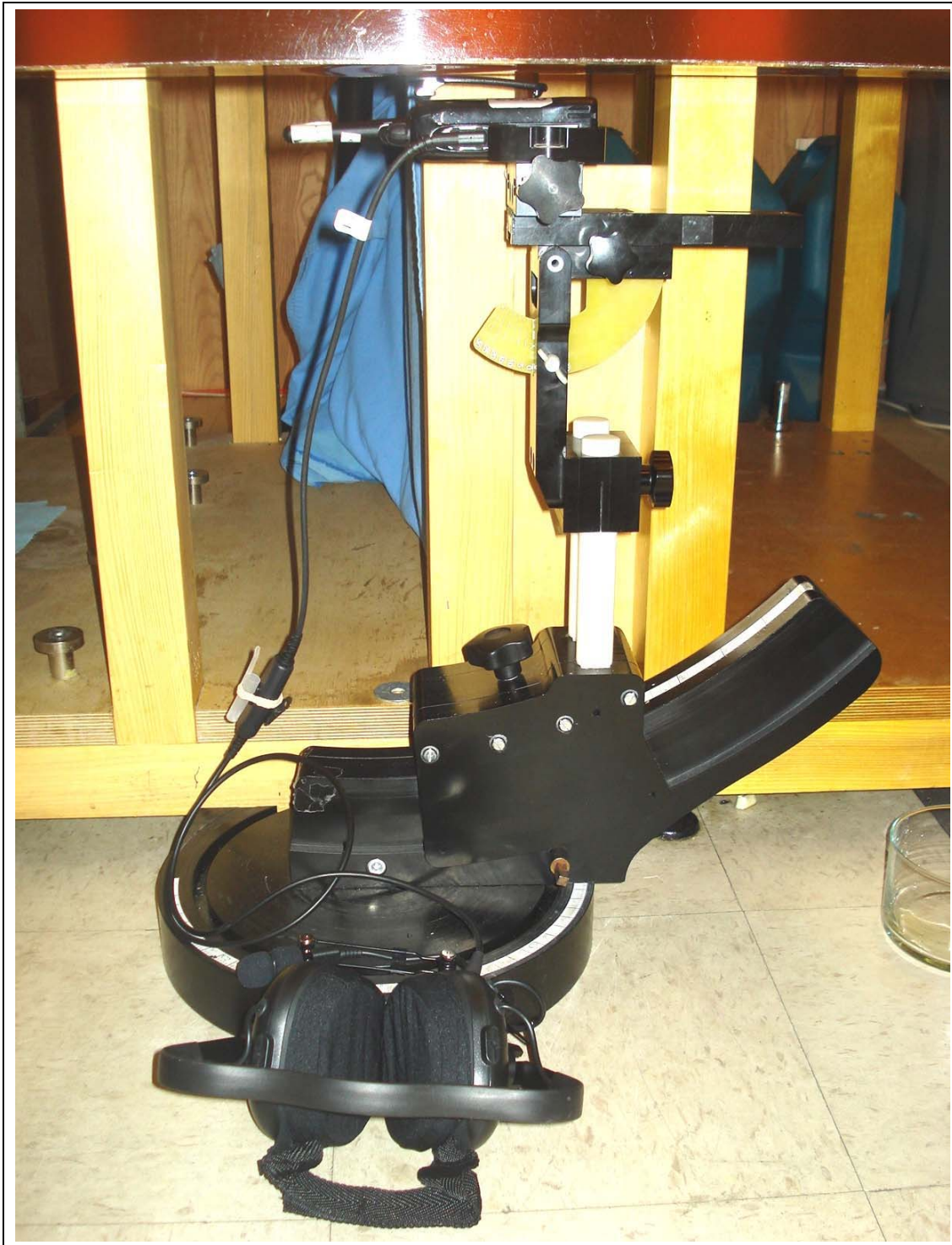
Body-worn SAR Test Setup with KBH-12 Belt-Clip and Default Audio Accessory (Headset P/N: KHS-10-BH)
