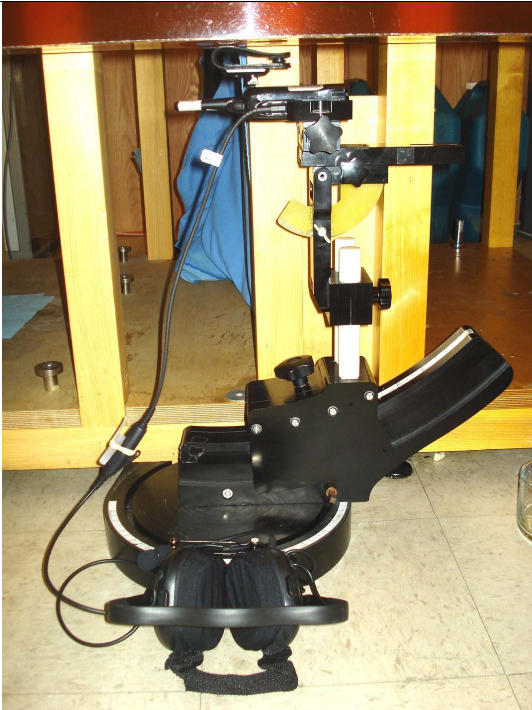
Body-worn SAR Test Setup with KBH-13DS Swivel Belt-Loop and Default Audio Accessory (Headset P/N: KHS-10-BH)
