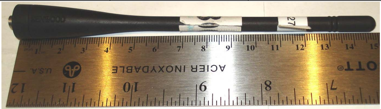
Detachable Whip "Antenna C" P/N: KRA-27M (Length = 149 mm)
