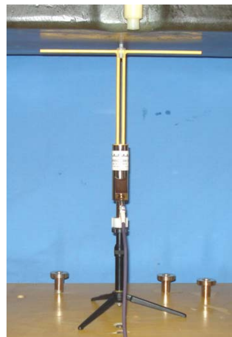
SPEAG 450 MHz Validation Dipole Setup
