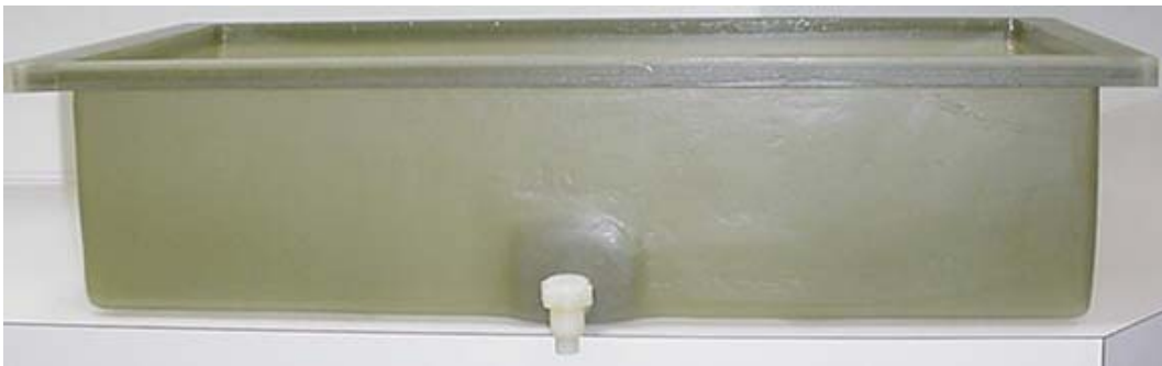
Fiberglass Planar Phantom - Front View
