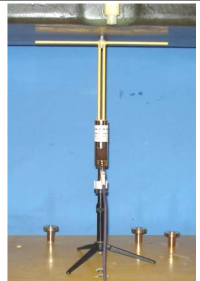
SPEAG 450 MHz Validation Dipole Setup
