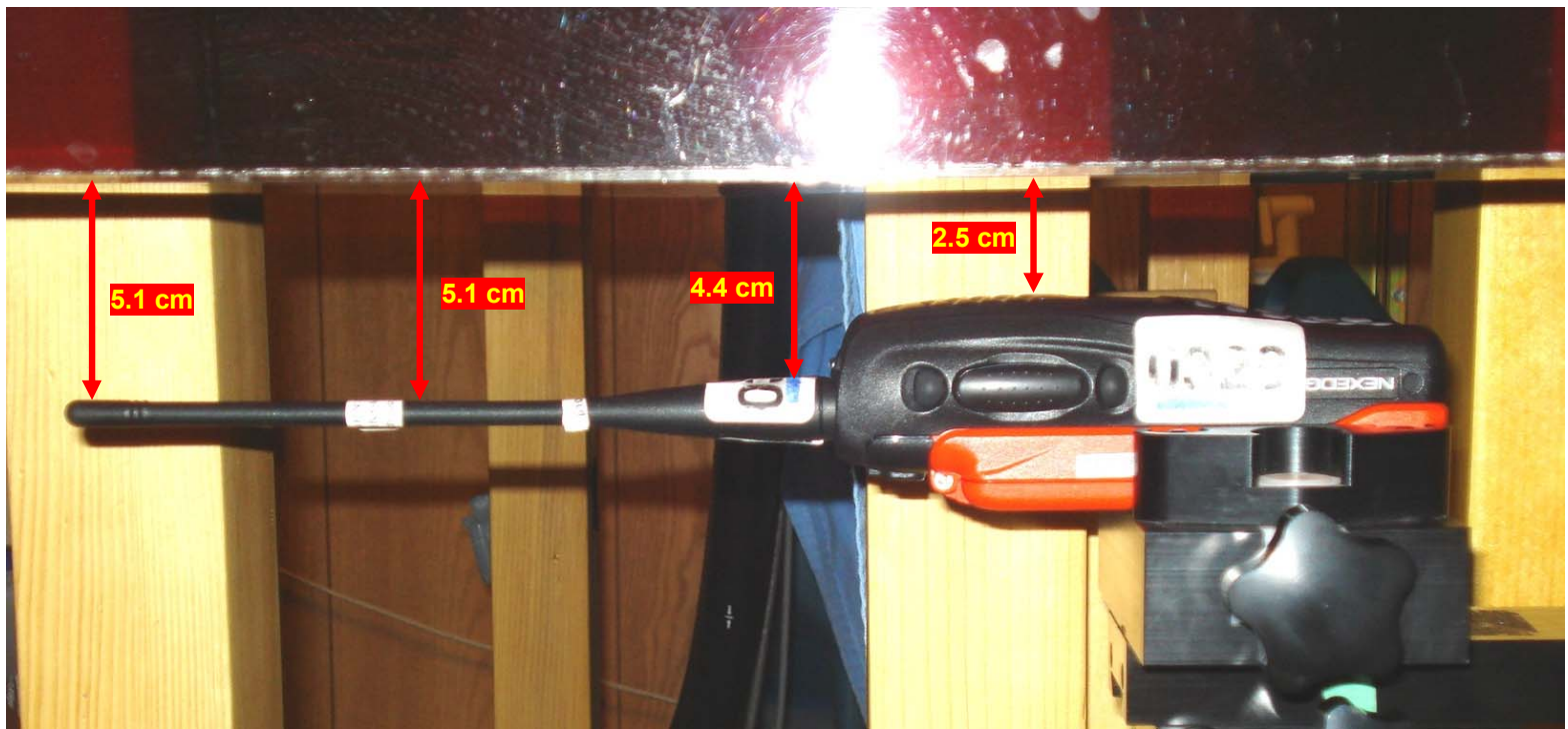
ANTENNA A - Face-held Test Setup with KRA-32 Whip Antenna & Alkaline Battery Case "c"
