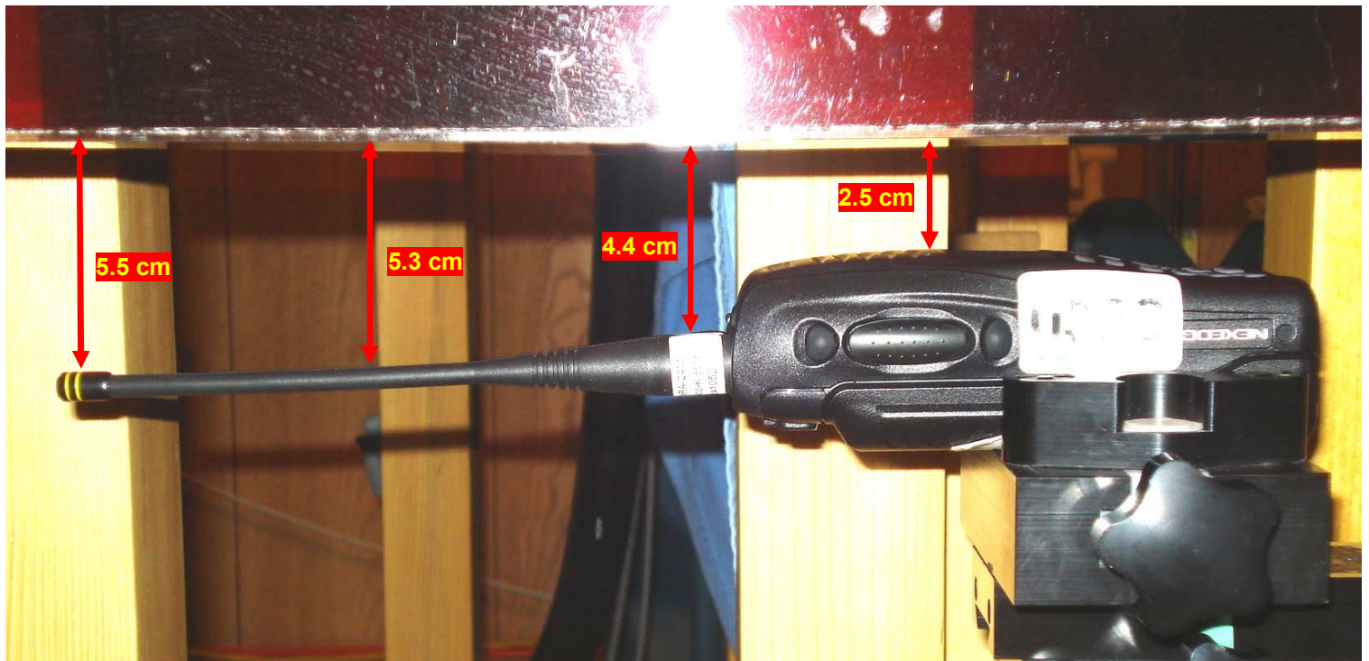
ANTENNA B - Face-held Test Setup with KRA-24M Whip Antenna & Ni-MH Battery "b"
