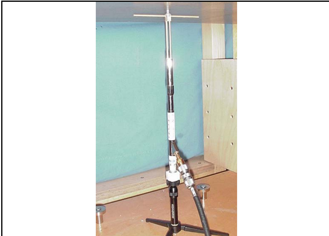
835 MHz SPEAG Validation Dipole Setup with Barski Planar Phantom
