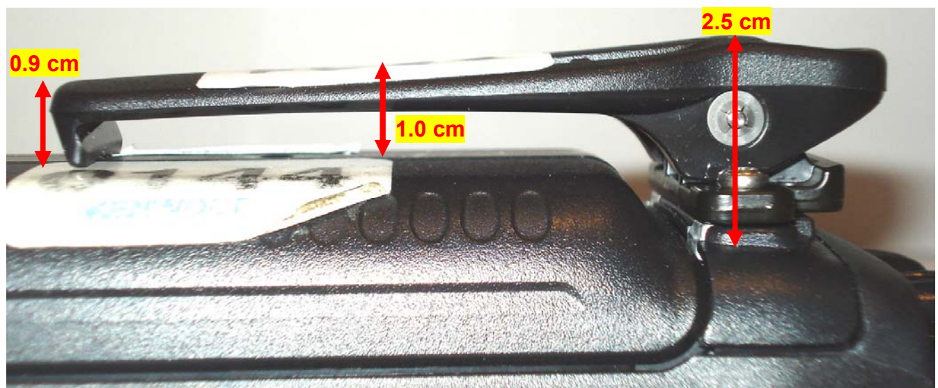
Belt-Clip Thickness Measurement Distance – Radio with Ni-MH Battery “b”
