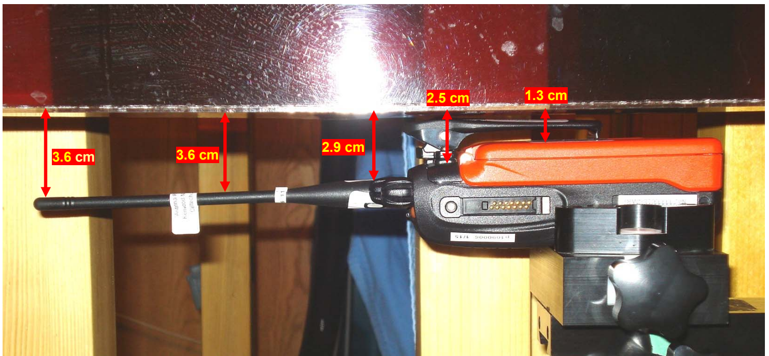
ANTENNA A - Body-worn Test Setup with KRA-32 Whip Antenna & Alkaline Batt Case "c" – 2.5 cm Belt-Clip Spacing - Battery Housing Parallel to Phantom
