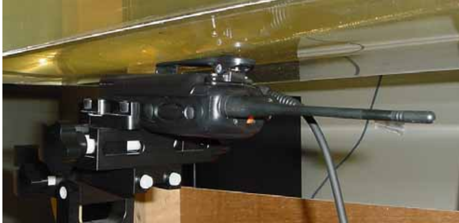
Body SAR with KRA-27M antenna, KBH-11 Belt Clip and Thick Battery
