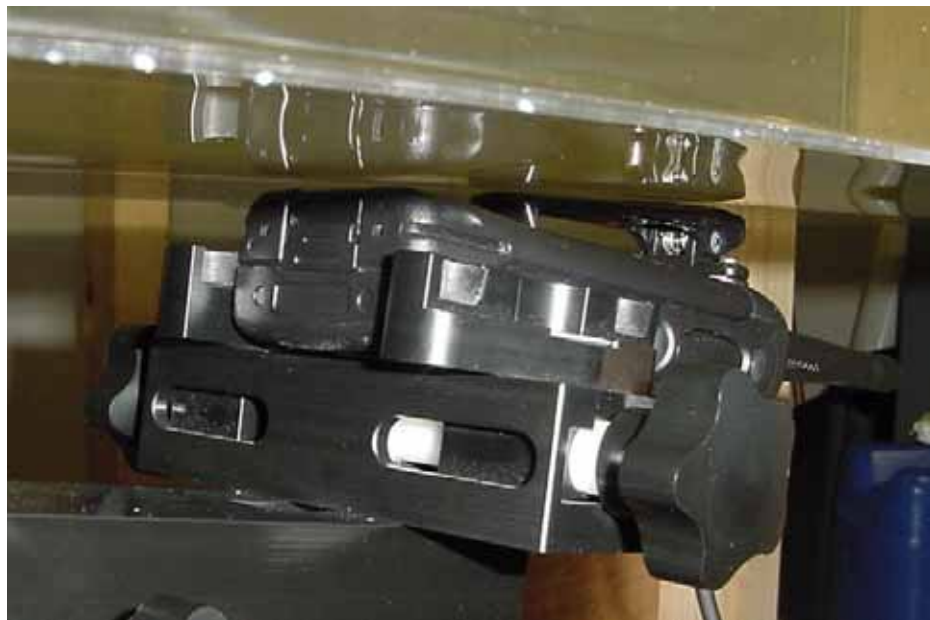
Body SAR with KRA-23M antenna, KBH-11 Belt Clip and Slim Battery
