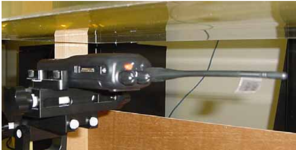
Face SAR with KRA-27M antenna and Thin Battery
