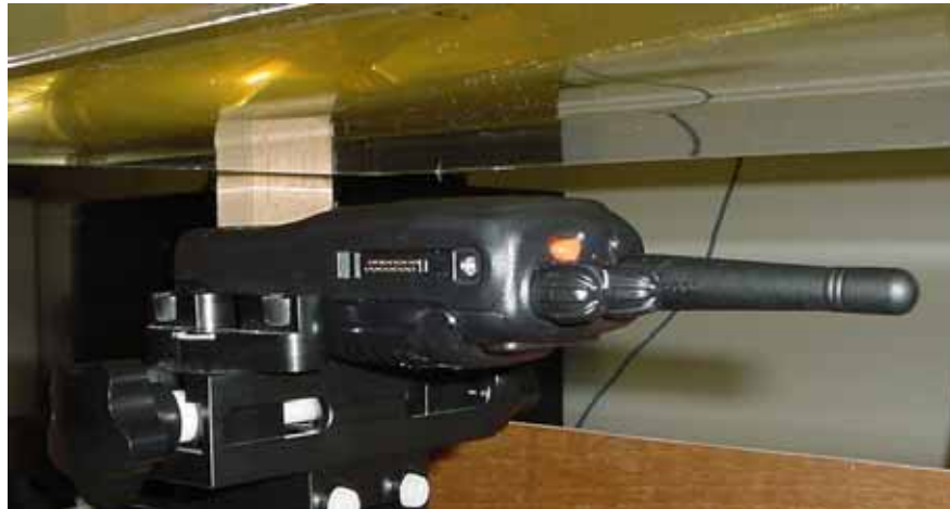
Face SAR with KRA-23M antenna and Thick Battery
