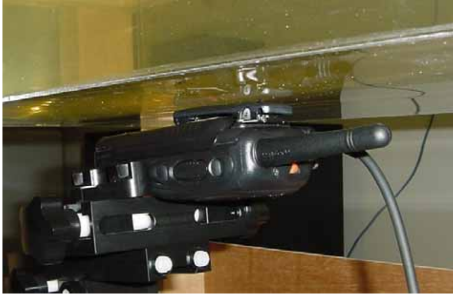
Body SAR with KRA-23M antenna, KBH-10 Belt Clip and Thick Battery
