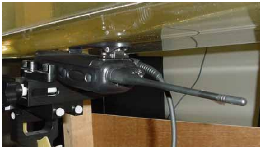
Body SAR with KRA-27M antenna, KBH-11 Belt Clip and Slim Battery
