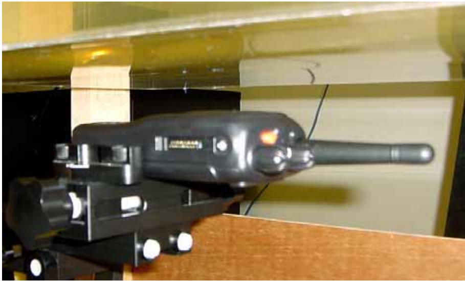
Face SAR with KRA-23M antenna and Slim Battery
