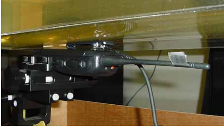
Body SAR with KRA-27M antenna, KBH-10 Belt Clip and Slim Battery
