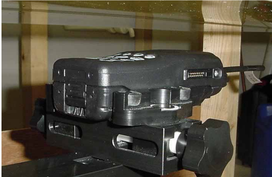
Face SAR with KRA-27M antenna and Thick Battery Style
