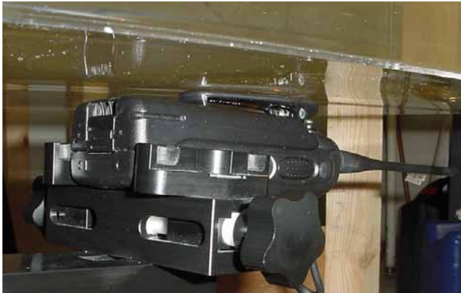
Body SAR with KRA-27M antenna, KBH-11 Belt Clip and Thick Battery
