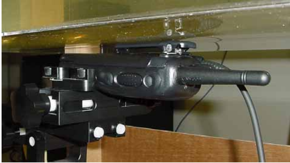
Body SAR with KRA-23M antenna, KBH-10 Belt Clip and Slim Battery
