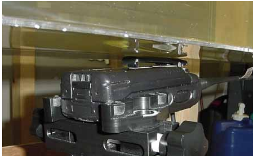
Body SAR with KRA-27M antenna, KBH-10 Belt Clip and Thick Battery
