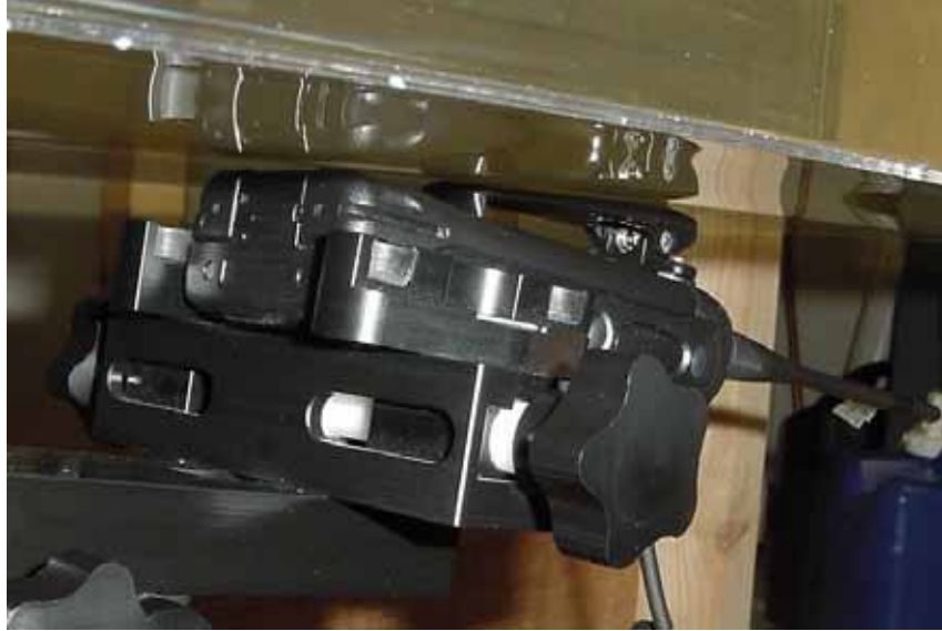
Body SAR with KRA-27M antenna, KBH-11 Belt Clip and Slim Battery
