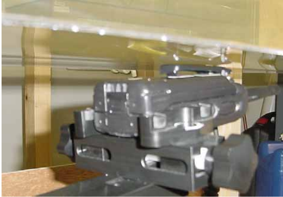
Body SAR with KRA-23M antenna, KBH-10 Belt Clip and Thick Battery
