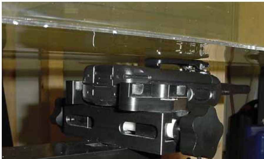
Body SAR with KRA-23M antenna, KBH-10 Belt Clip and Slim Battery
