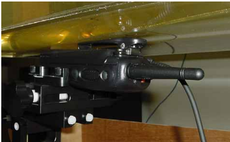
Body SAR with KRA-23M antenna, KBH-10 Belt Clip and Thick Battery
