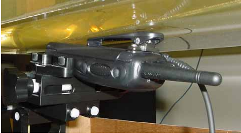
Body SAR with KRA-23M antenna, KBH-11 Belt Clip and Slim Battery
