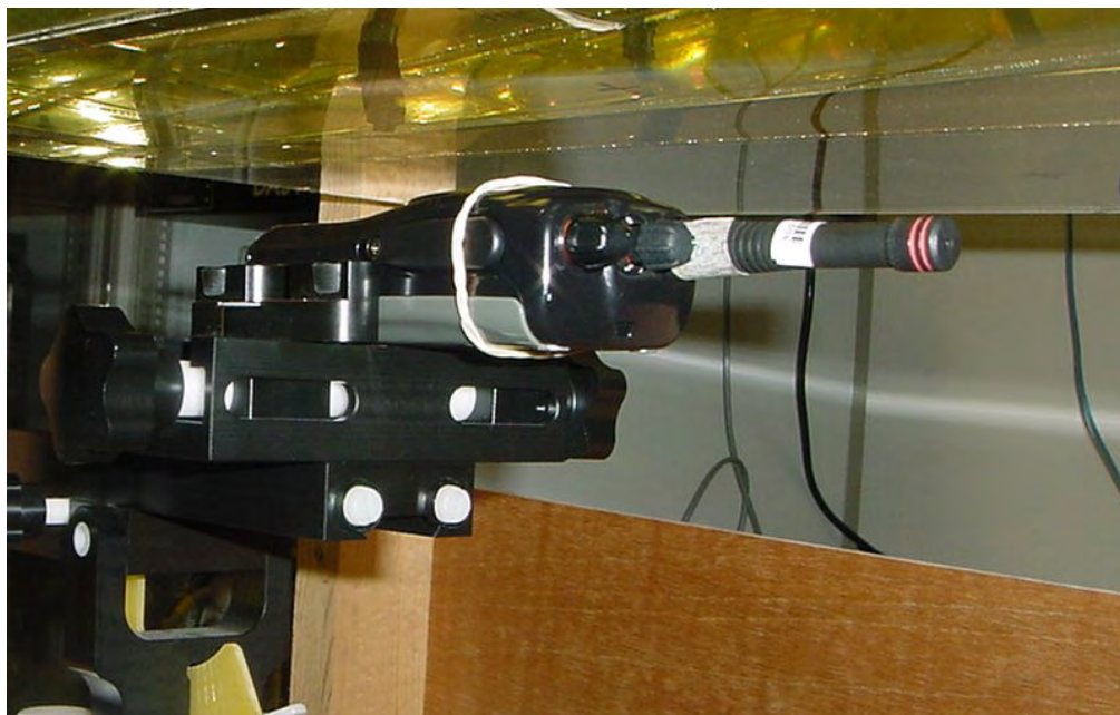
Photograph 5. Face Held at 2.5cm Separation with Stubby Antenna
