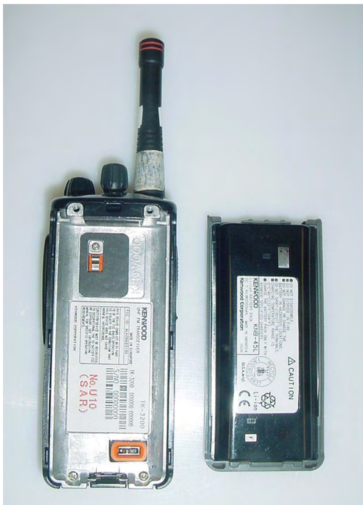
Photograph 9. Exploded View of TK-3200 and KNB-45L Battery
