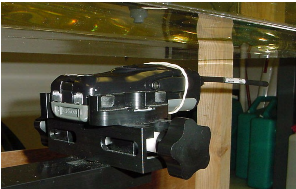
Photograph 8. Face Held at 2.5cm Separation with Whip Antenna
