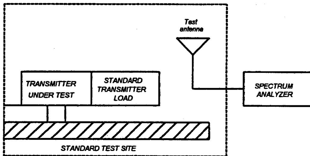
**Name of Test:** Field Strength of Spurious Radiation (Cont.)
