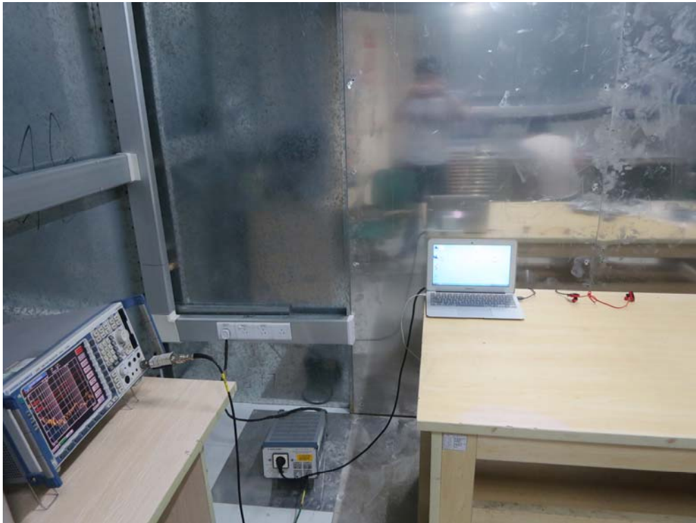
FCC RADIATED EMISSION TEST SETUP
