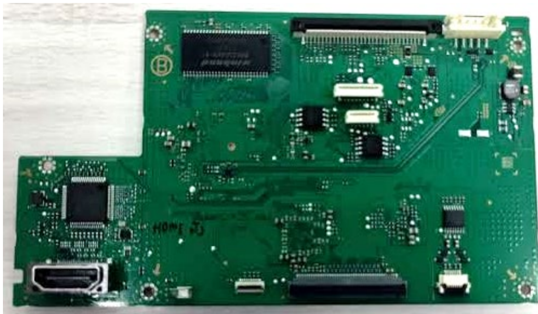
Display PWB(Front Side)
