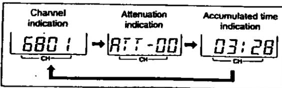
In Attenuation indication mode, it displays the input attenuation setting in dB, which can be changed in a range of 0 to 21 dB in 3-dB steps.
