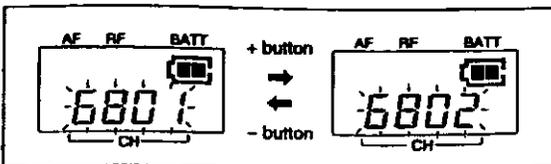
If you keep either button pressed, the channel setting will be incremented or decremented successively. The display will cycle from 68-01 through 69-47.
