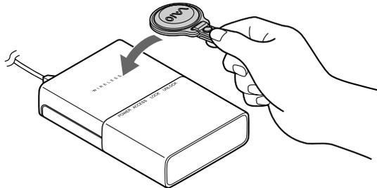
The LOCK and UNLOCK indicators flash alternately, then the wireless key is registered to the drive.
