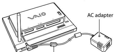
The ferrite core is supplied with U.K. model only.
