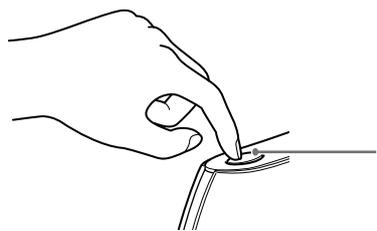
Press and hold the AOSS button until the access point indicator blinks.
