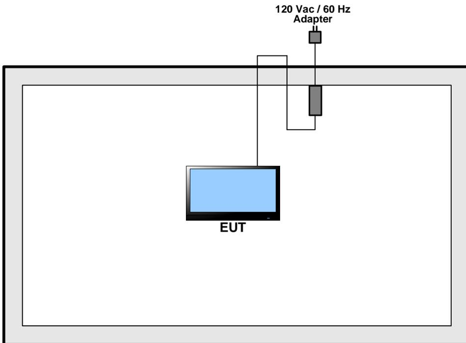
For radiated emissions 30MHz~1GHz
