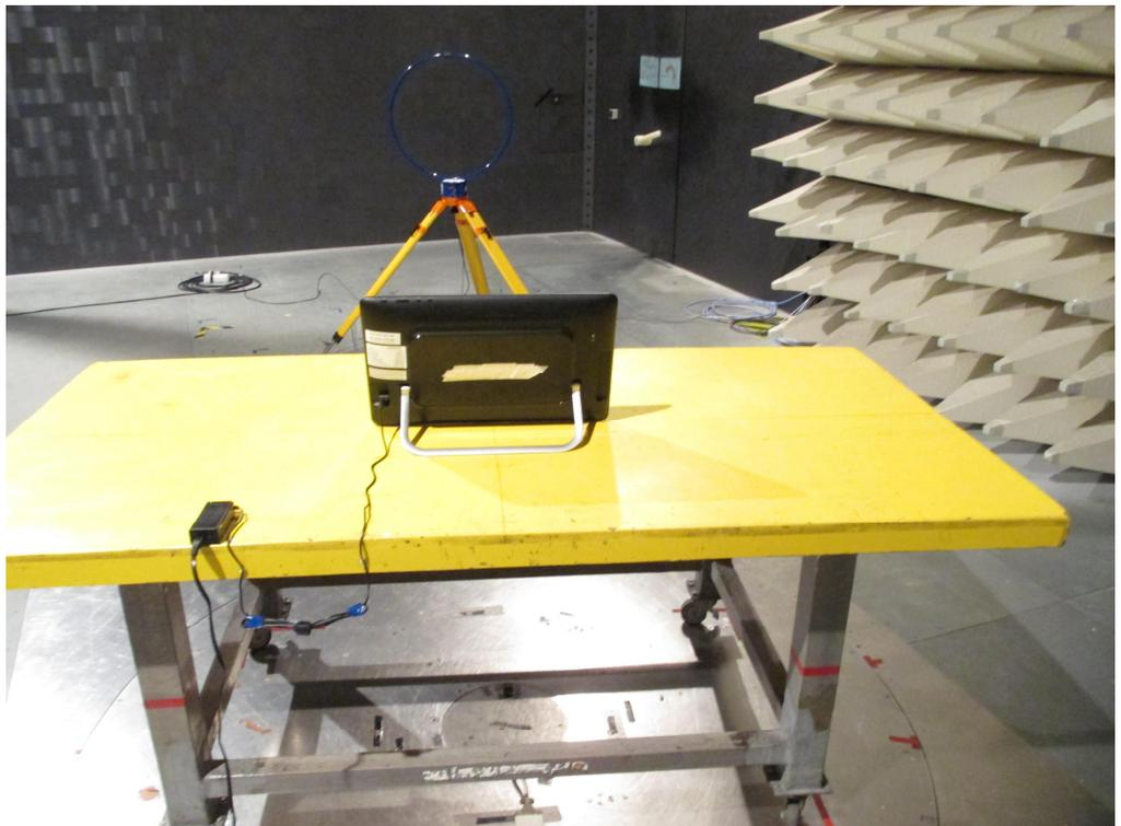
For radiated emissions 30MHz~1GHz
