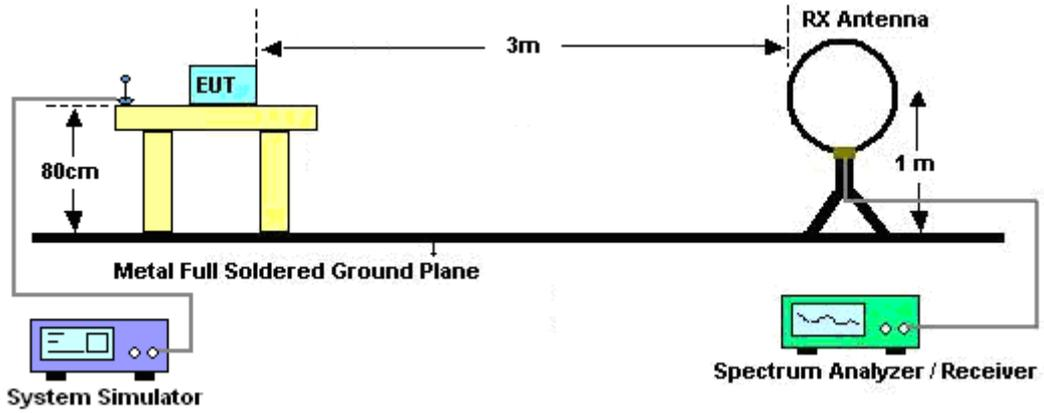
For radiated emissions from 30MHz to 1GHz
