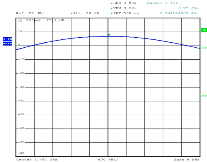
Peak Output Power Plot on Channel 78
