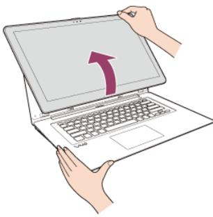
4. Move the LCD screen in the direction of the arrow to fold the screen. The LCD screen is folded on the keyboard.
