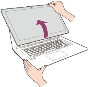
4. Move the LCD screen in the direction of the arrow to fold the screen.
