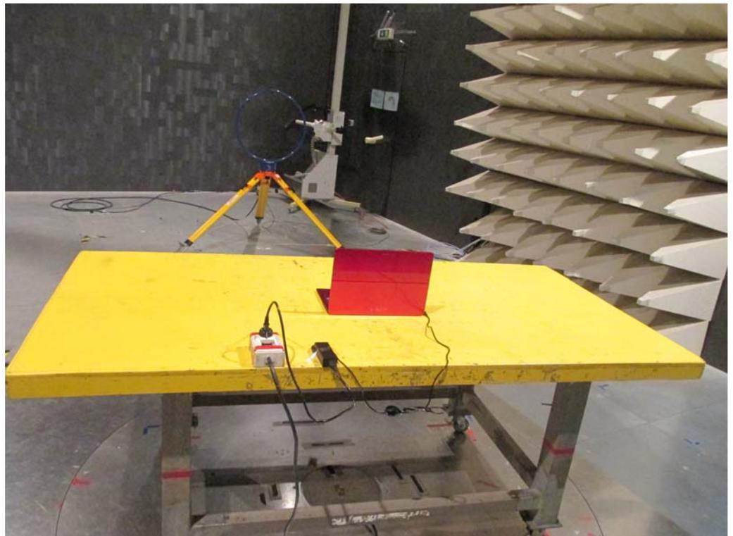
Test Configuration: 30MHz~1GHz / Test Mode: Mode 1
